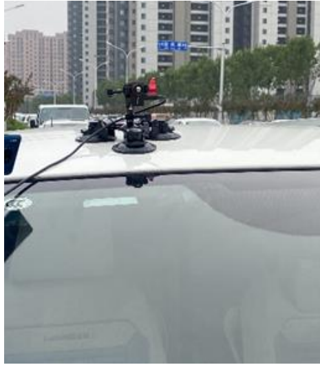
Figure 15 - Far infrared camera installation position
