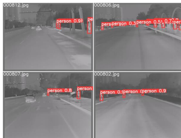
Figure 31 - The pedestrian detection effect verification diagram of the model before the introduction of the SE module
