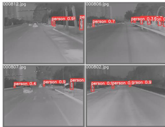
Figure 31 - The pedestrian detection effect verification diagram of the model before the introduction of the SE module
