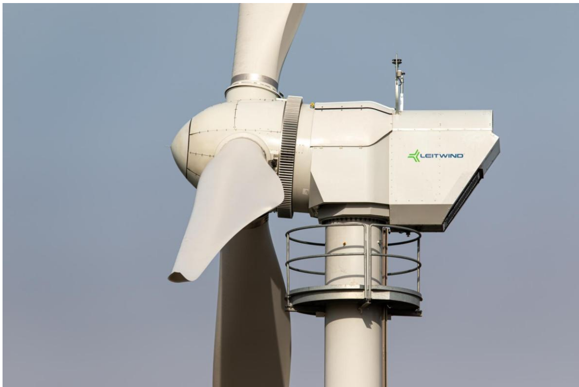
Figure 3 Shows the Leitwind LTW42 250kW wind turbine
