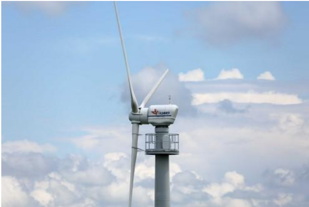
Figure 2 Shows the Hummer H25.0-200kW wind turbine.
