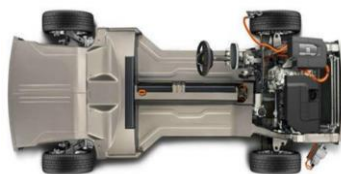
Figure 2-5: Chevrolet Volt Battery Pack
