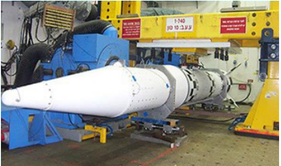
Figure 11 Large Scale Assembled Munition under Vibration Testing
