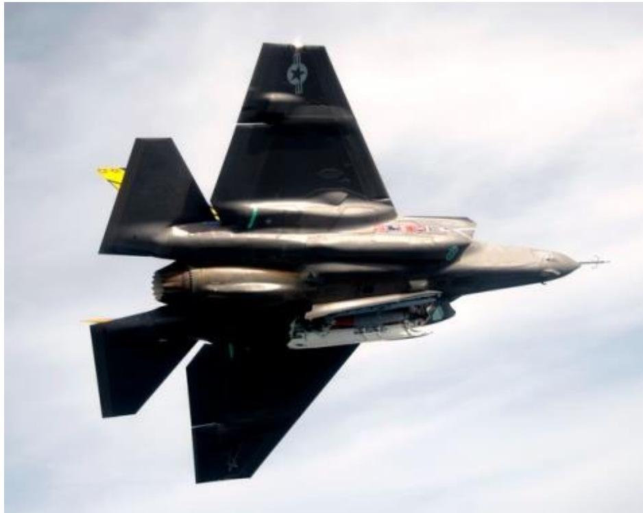
Figure 1 F-35 Lightning displaying its internal weapons bay
