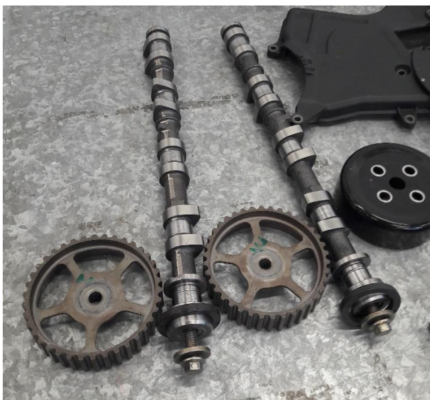
Figure 2 - Picture showing camshafts and camshaft pulleys.
