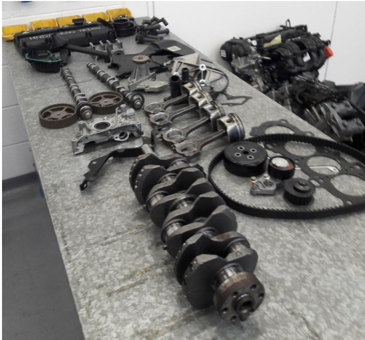
Figure 7 - Picture showing all parts removed from the engine block.
