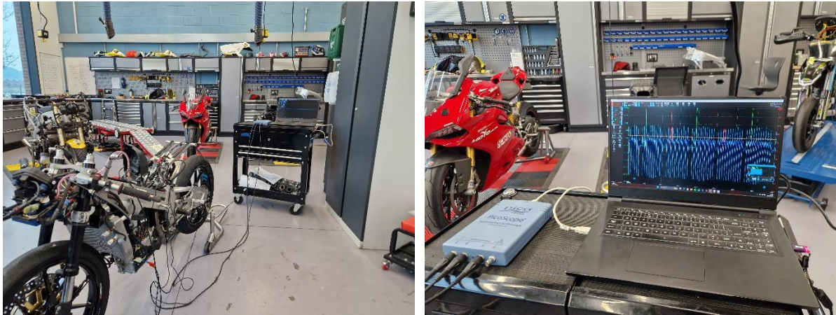
Figure 56: Pico scope setup for recording engine component electrical traces.
