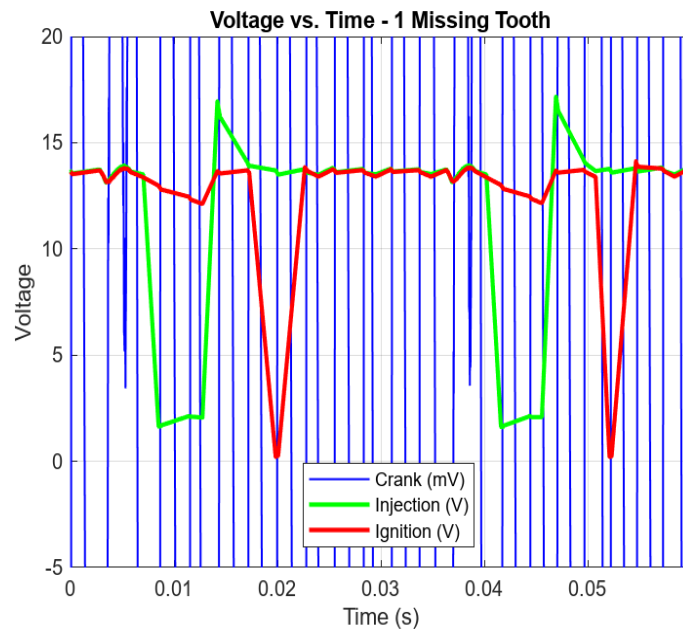
Figure 8: Corrected crank trigger trace.
