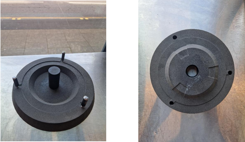
Figure 15: Forming tool base (left), top (right).
