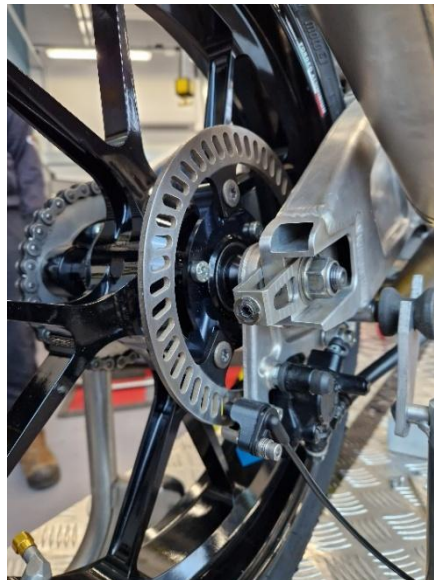
Figure 17: Rear disc mild steel prototype.
