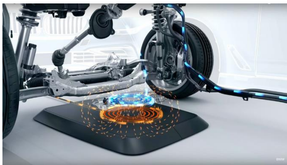
Figure 72 Volvo Wireless Charging production development (Moldrich, 2022)
