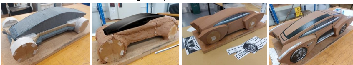
Figure 52 Photos of the Jaguar GT Clay Model from Body Buck - adding Decals and Details (Burton, Matthews, Shelton, Henwood 2022)
