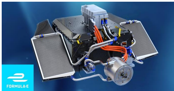
Figure 55 Formula E Engine Powertrain Unit (ABB Formula E, 2017)
