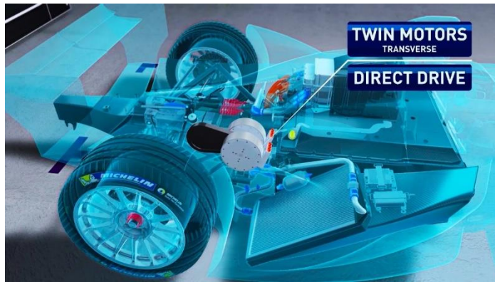
Figure 56 Formula E 2 Motor Gear Box (ABB Formula E, 2016)
