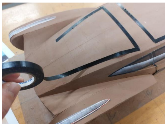
Figure 130 Masking tape outline for decals and applying details of tape and spoiler to my model (Burton, 2022)
