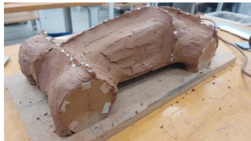
Figure 123 Outlining the clay structure of how much clay is needed (Burton, 2022)
