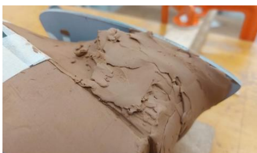
Figure 126 Defining the sides and body volume before defining the wheel pods (Burton, 2022)
