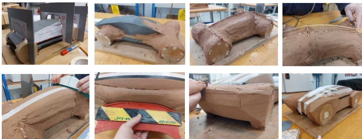
Figure 63 Photos of the Clay model from Start to Finish (Burton, Matthews, Shelton, 2022)
