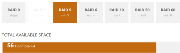
Figure 32: Results from RAID 5 calculator for 64TB of storage. Source: [44].
