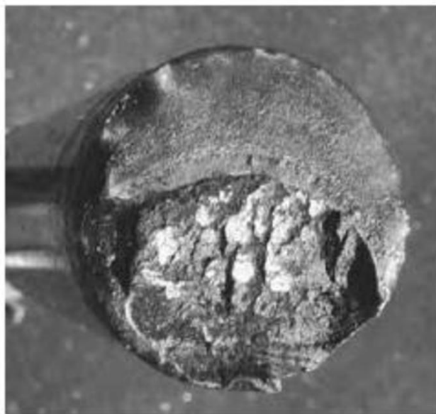
Figure 4 - Driveshaft Failure, Rogers, K. (2026)
