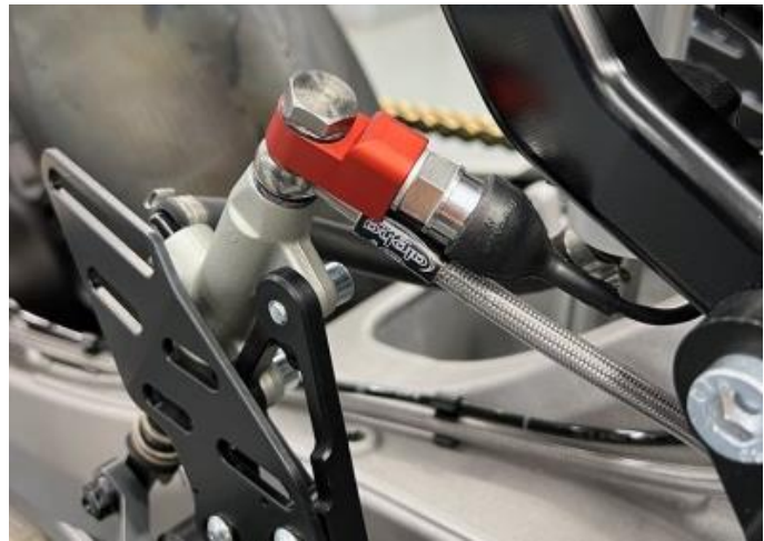
Figure 11 Rear Brake Pressure sensor from 2D (MRTTECH, 2026)
