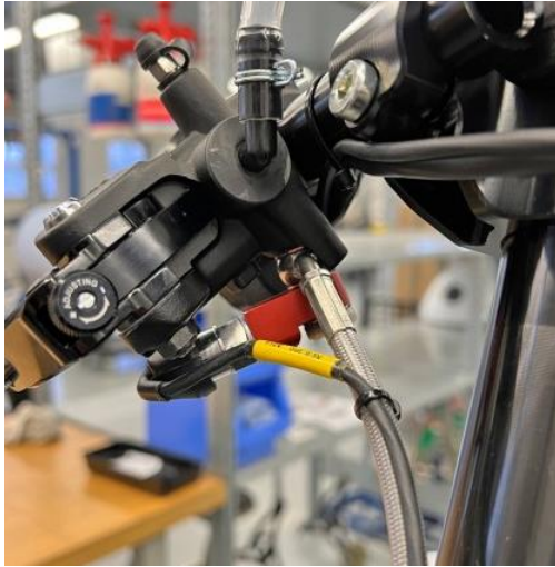
Figure 10 Front Brake Pressure sensor from 2D (MRTTECH, 2026)
