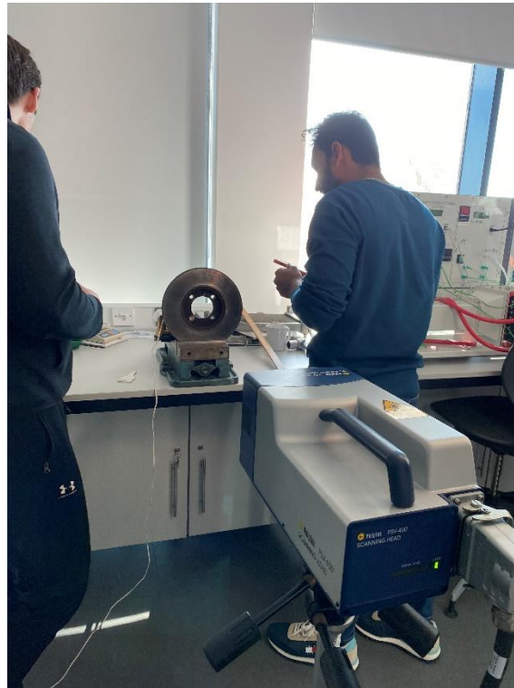
Fig. 2: PolyTec Scanning Laser Doppler Vibrometer Placed in Front of the Brake Disc
