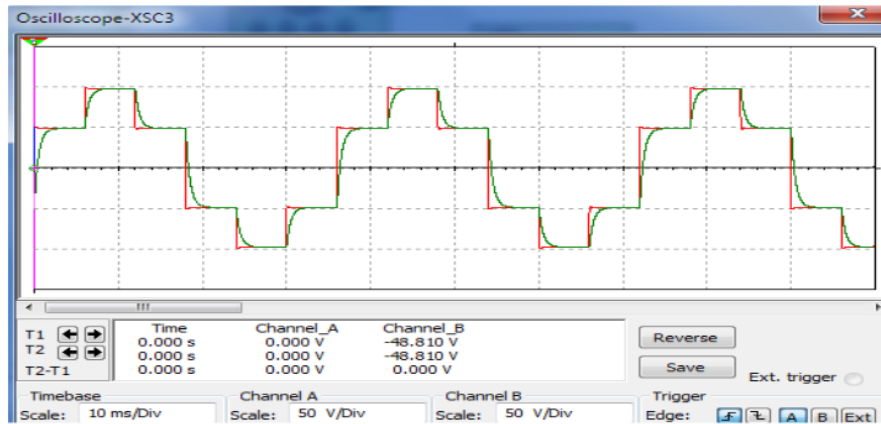
Figure 19- output waveform with motor inductance
