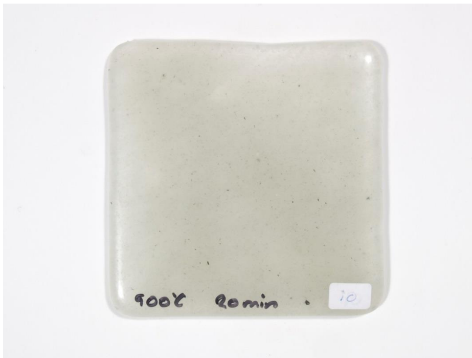
Figure 10: Contaminated Recycled Glass Tile (Oseng, 2009)
