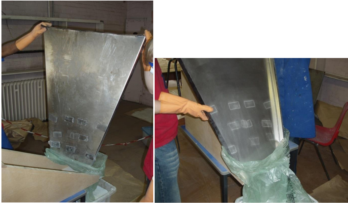
Figure 11: Magnets on Steel Sheet and Figure 12: Contaminant Removed by Magnets (Oseng, 2009)
