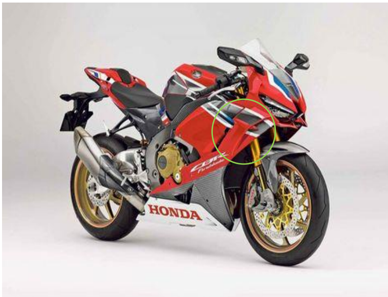
Figure 5: 2019 CBR with front wings (Honda Global)
