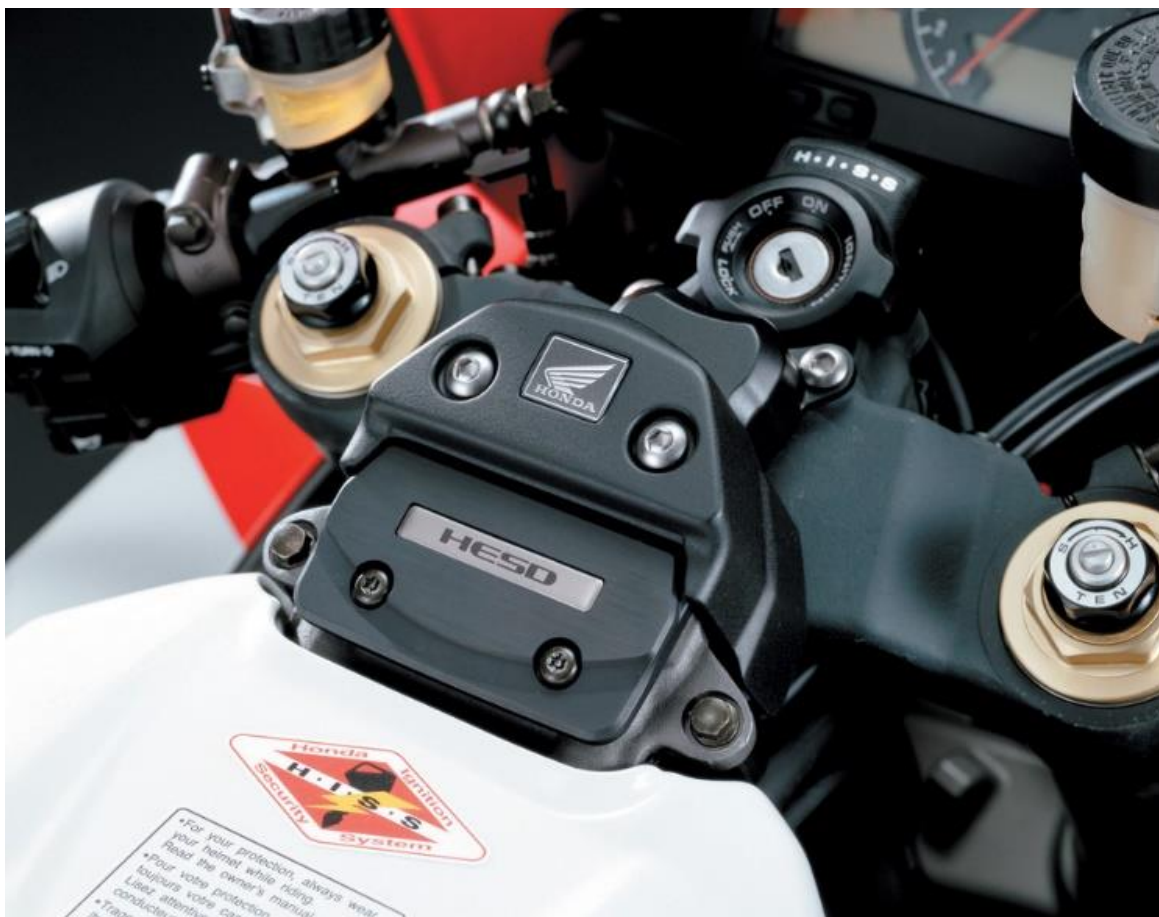
Figure 9: HESD on 2004 CBR1000RR (American Honda Motor Co.)
