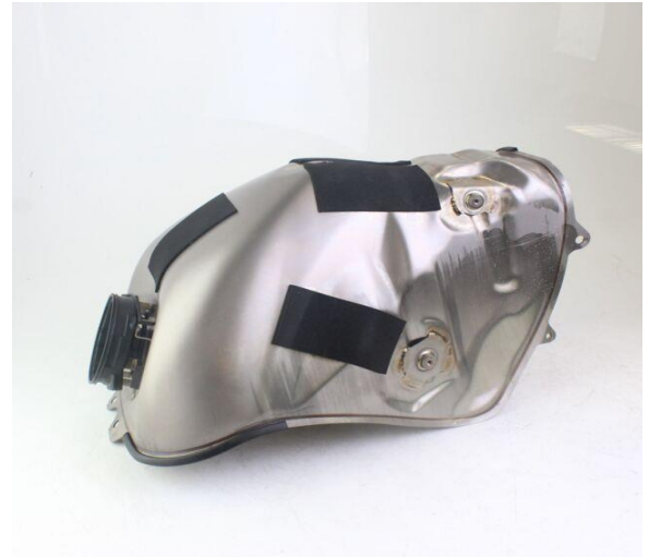
Figure 6: 2019 CBR titanium fuel tank (surreymcparts)
