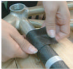
PREPREG COMPOSITE IS LAID-UP BY HAND
