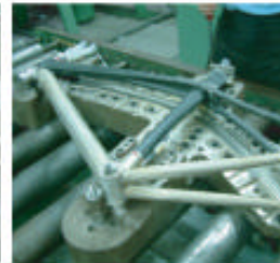
CURED CO-MOLDED MONOCOQUE FRAME IS REMOVED FROM THE MOLD FOR HAND FINISHING
