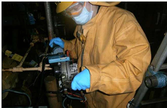
Figure 5 Disconnecting air supply
