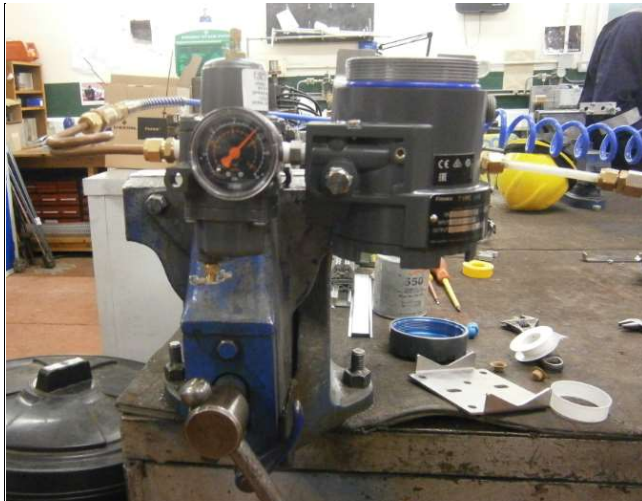
Figure 9 New I to P calibration setup
