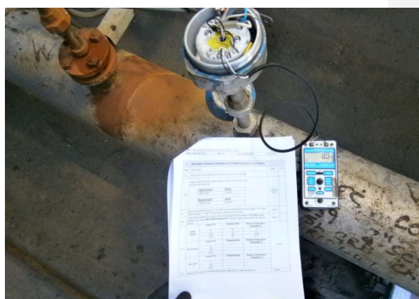
Figure 4 Calibrator connected, checking procedure
