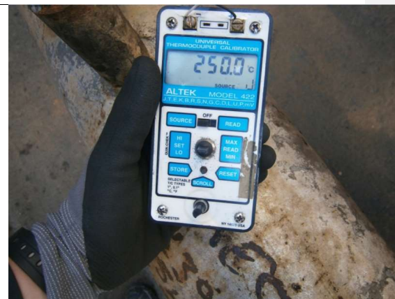
Figure 7 Temperature calibrator 250C
