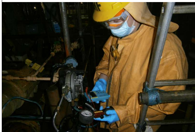
Figure 6 Connecting hand pump
