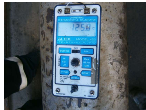
Figure 5 Temperature calibrator 125°C
