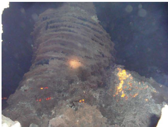
Figure 1.6b Cohesive zone after blow-down
