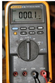
Figure 20: Multi Meter reading on earth bonding resistance check
