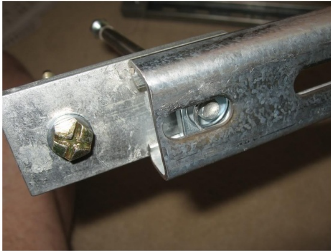
Figure 18: As can be seen, spring washers, nuts and bolts have been used to construct the bracket. All came at no extra cost as these spares are kept on site.
