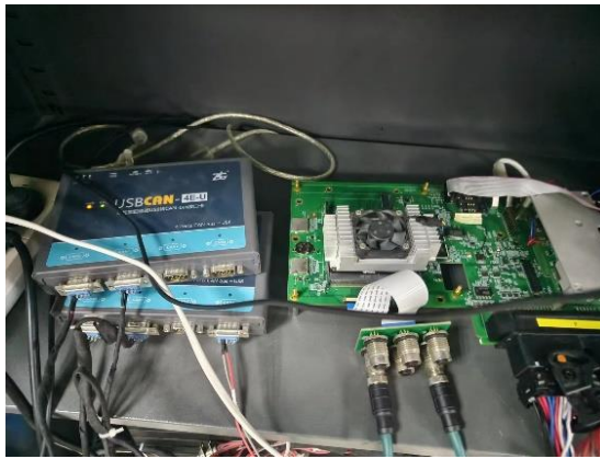
Figure 17 Controller and USB to CAN interface card Figure 18 Simulation operation interface
