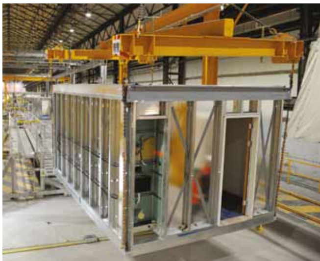
Light steel framed module
