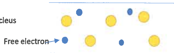
Fig 3. Insulator at high temperature
