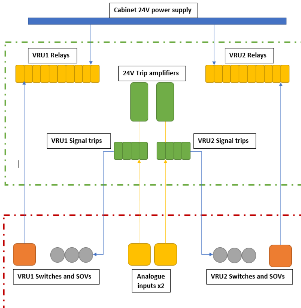
Figure 9: Relay and trip amplifier solution design
