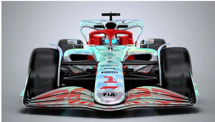
Figure 8 - 2022 FORMULA ONE Multi-Element Front Wing (Newbon, 2021)
