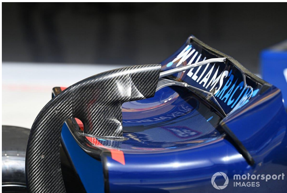
Figure 10 - Rear Wing and DRS actuator on the Williams FW44 (Sutton, 2022)
