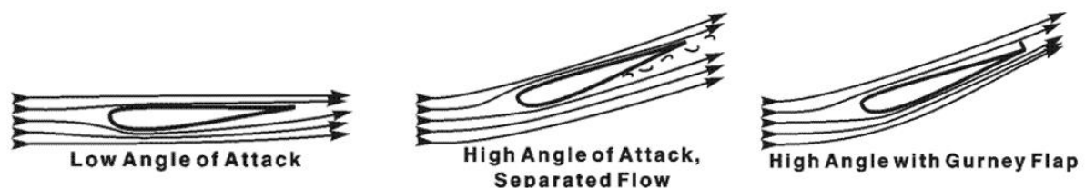
Figure 9 - Diagram showing effect of Gurney flap on aerodynamics of front wing (Formula 1 Dictionary, n.d.)
