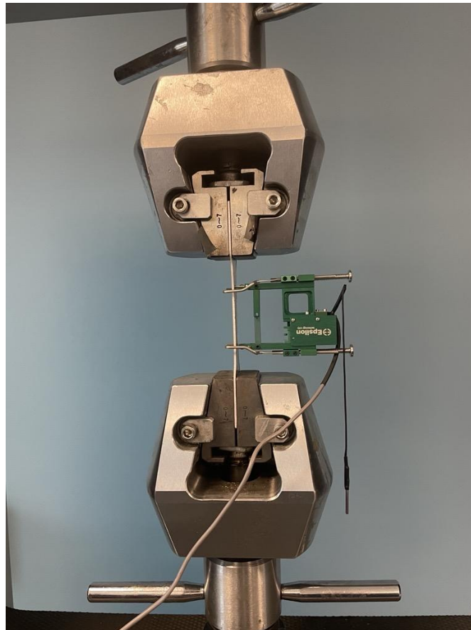
Figure 3 Aluminium sample set up in the Dennison machine with the extensometer attached
