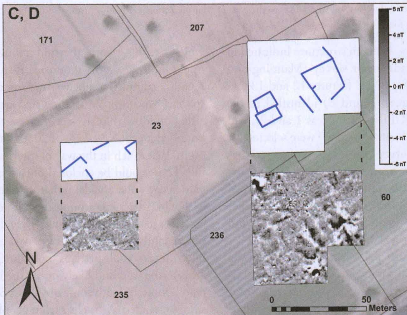
Figure 10. Detail of fluxgate gradiometer survey Blocks C and D with interpretations of magnetic signal. Blue interpretations indicate low (negative) magnetic anomalies, while black interpretations indicate high (positive) magnetic anomalies. A small ground-truthing excavation in Block C (see Figure 4) showed a linear anomaly to be an LC field-wall.
