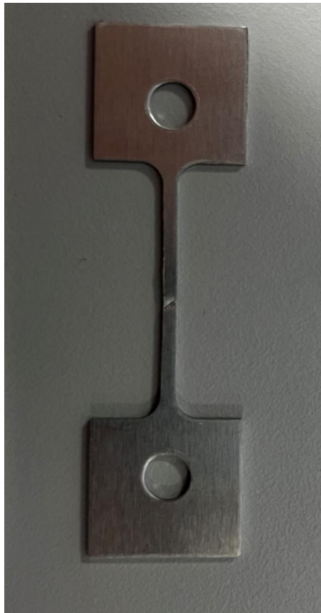
Figure 7 - Broken specimen with a small amount of Goose-necking
