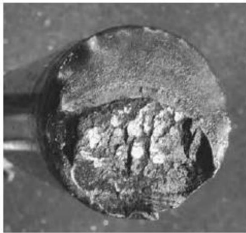
Figure 1 - Failure of Dakar Driveshaft (Rogers, 2026)
