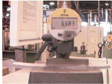
Figure 2.11 - (DTI) Dial test indicator Good detail
