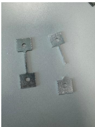
(Figure 4: Aluminium Alloy specimen before and after fracture)
