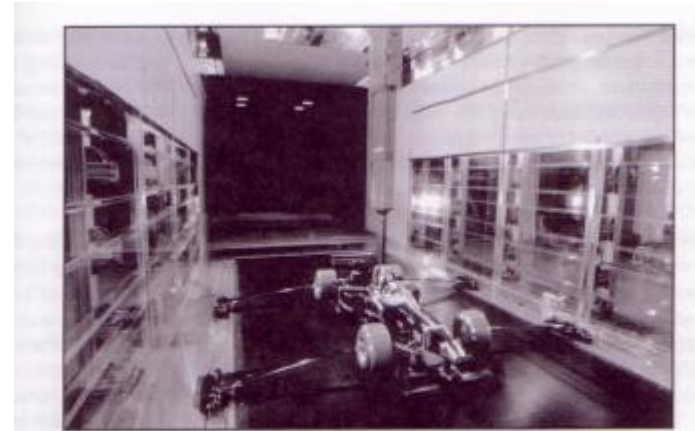
Fig. 8.3 Half-scale wind tunnel model mounted in wind tunnel. (Courtesy of Sutton Motorsport Images)
