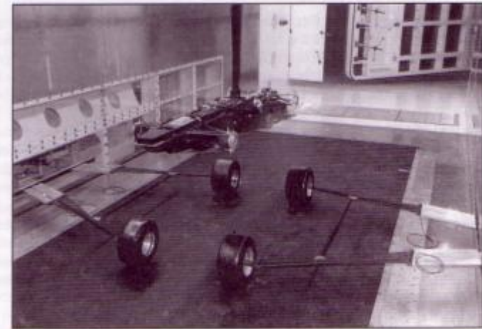
Fig. 8.4 Half-scale model without bodywork or wings fitted.
