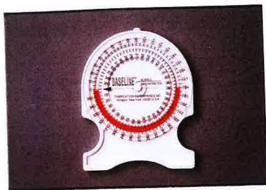
Figure 8.7a Start inclinometer dial at zero
