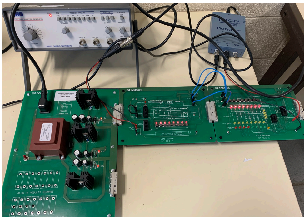
Figure 19 - Analog > Digital Convertor - Test Bench Setup
