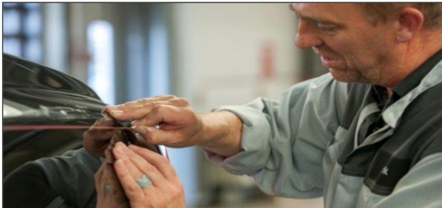
Figure 3.0 – Mark Court hand painting coach lines on a Rolls Royce vehicle.
