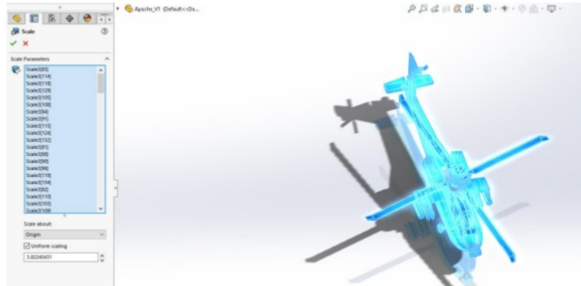
Figure 3. Scale feature on Solidworks (Solidworks, 2019)
