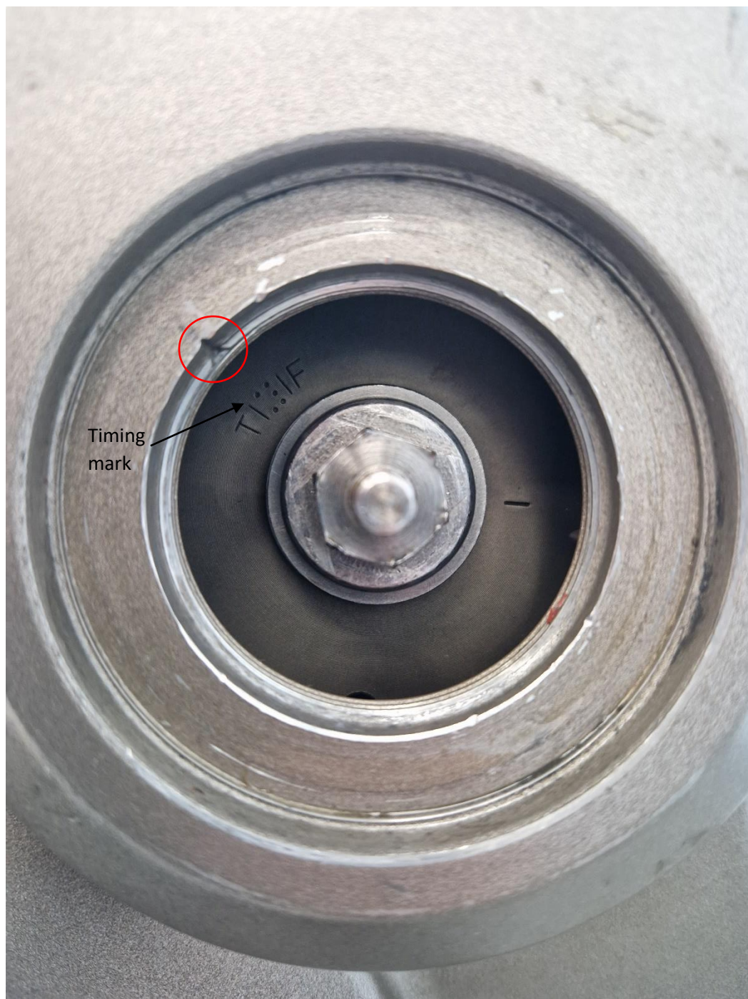
Figure 29: Timing mark on engine casing (red circle) and on engine internals.
