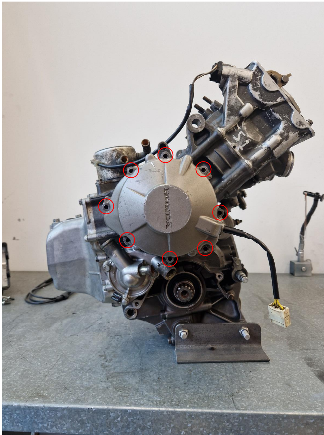
Figure 27: Stator cover bolt holes circled red.
