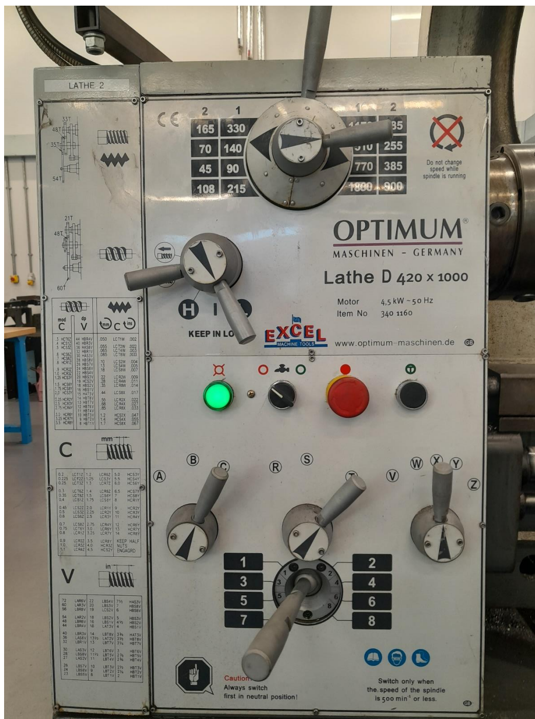
Figure 11: Lathe control panel showing green power light.
