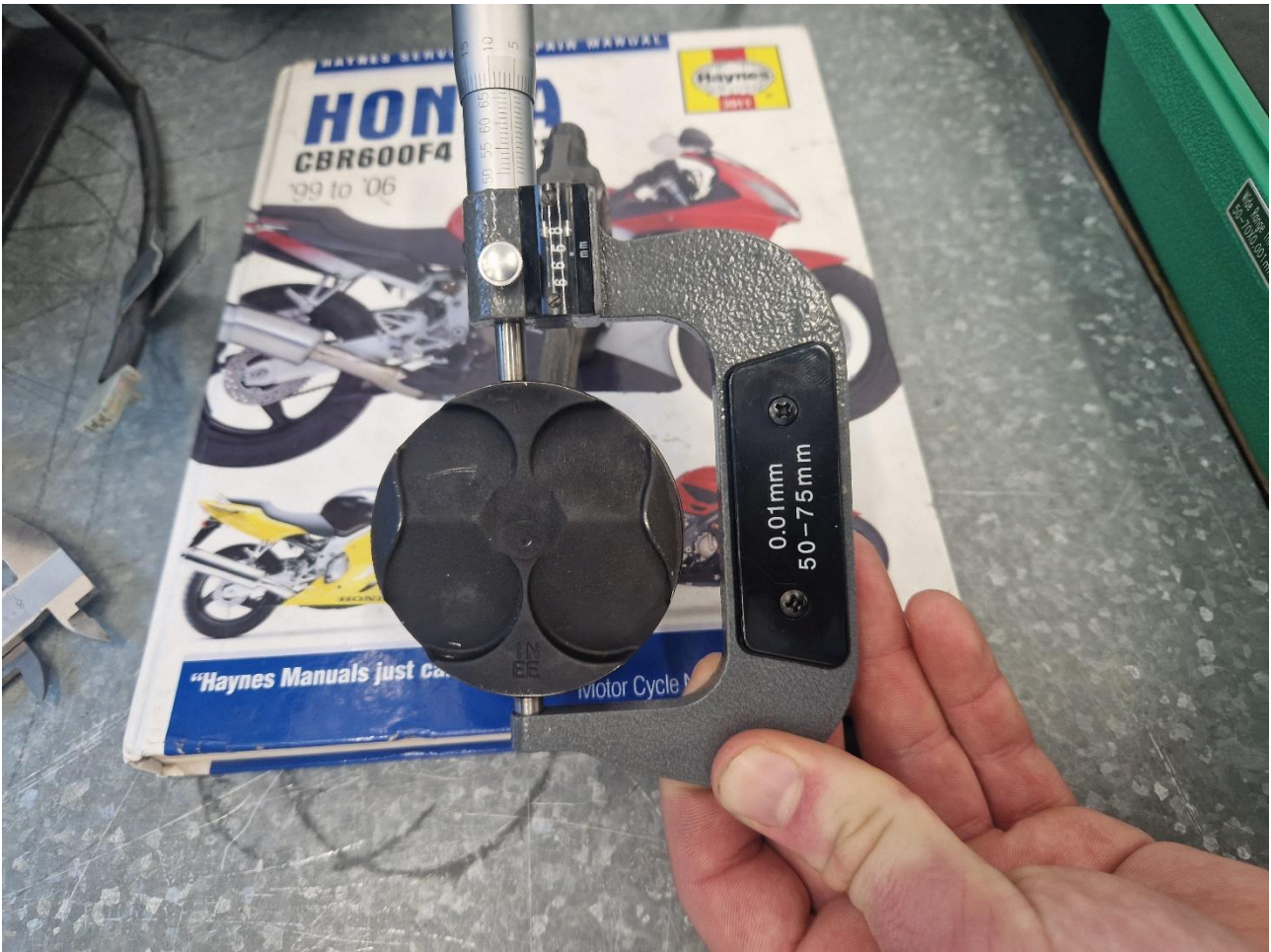
Figure 59: Front to back measurement of piston crown.
