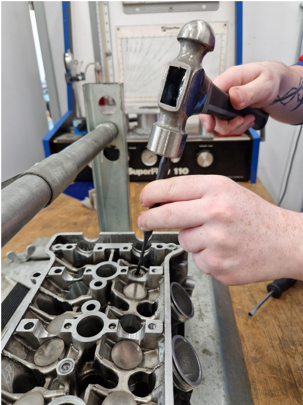
Figure 77: Ensuring collets have seated correctly.
