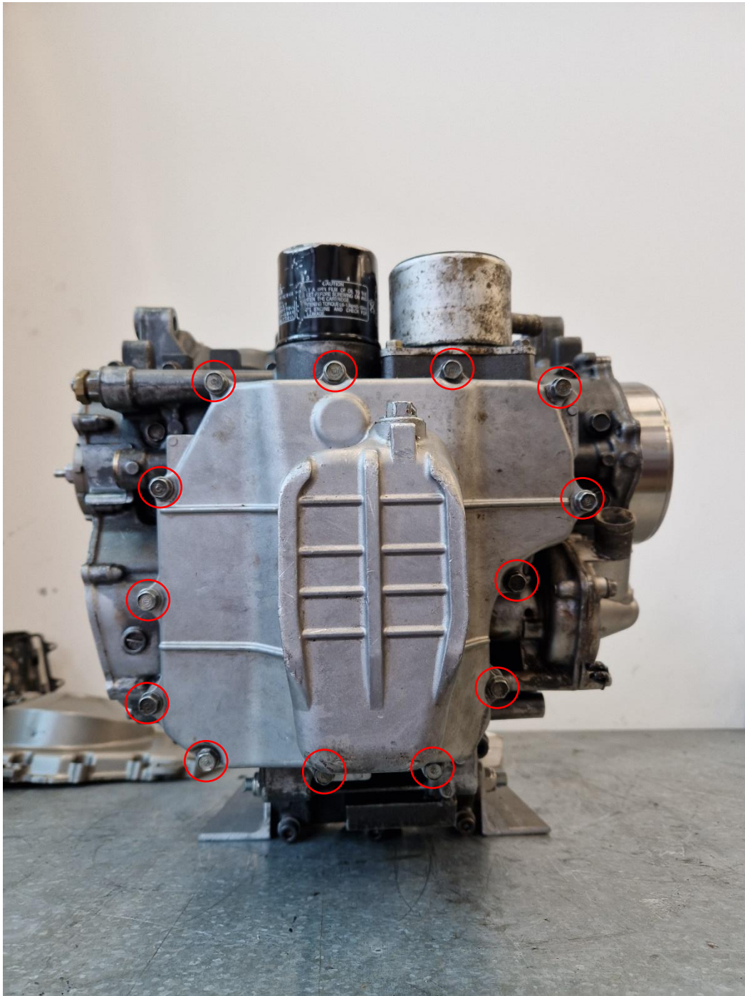
Figure 41: Sump bolts circled red.
