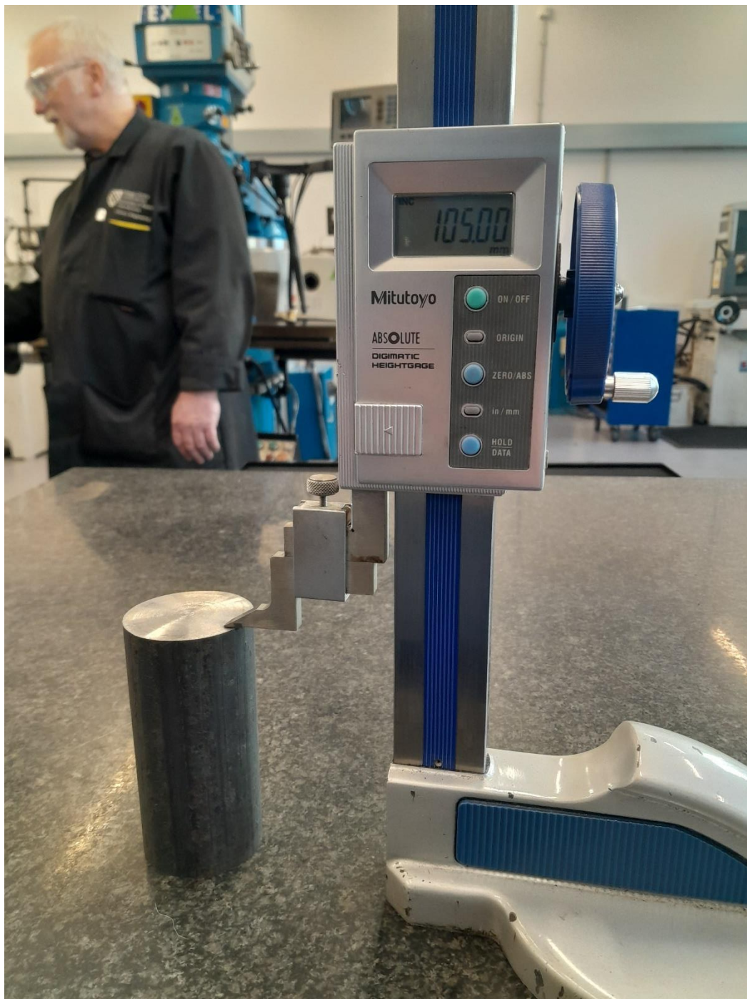
Figure 25: Measuring faced off work piece.
