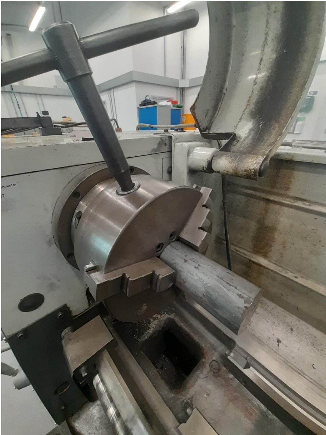
Figure 23: Work piece secured in vice jaws.
