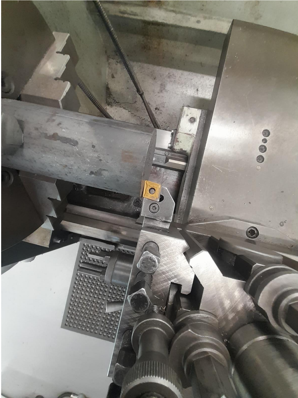
Figure 24: Cutting tool touch on with work piece.
