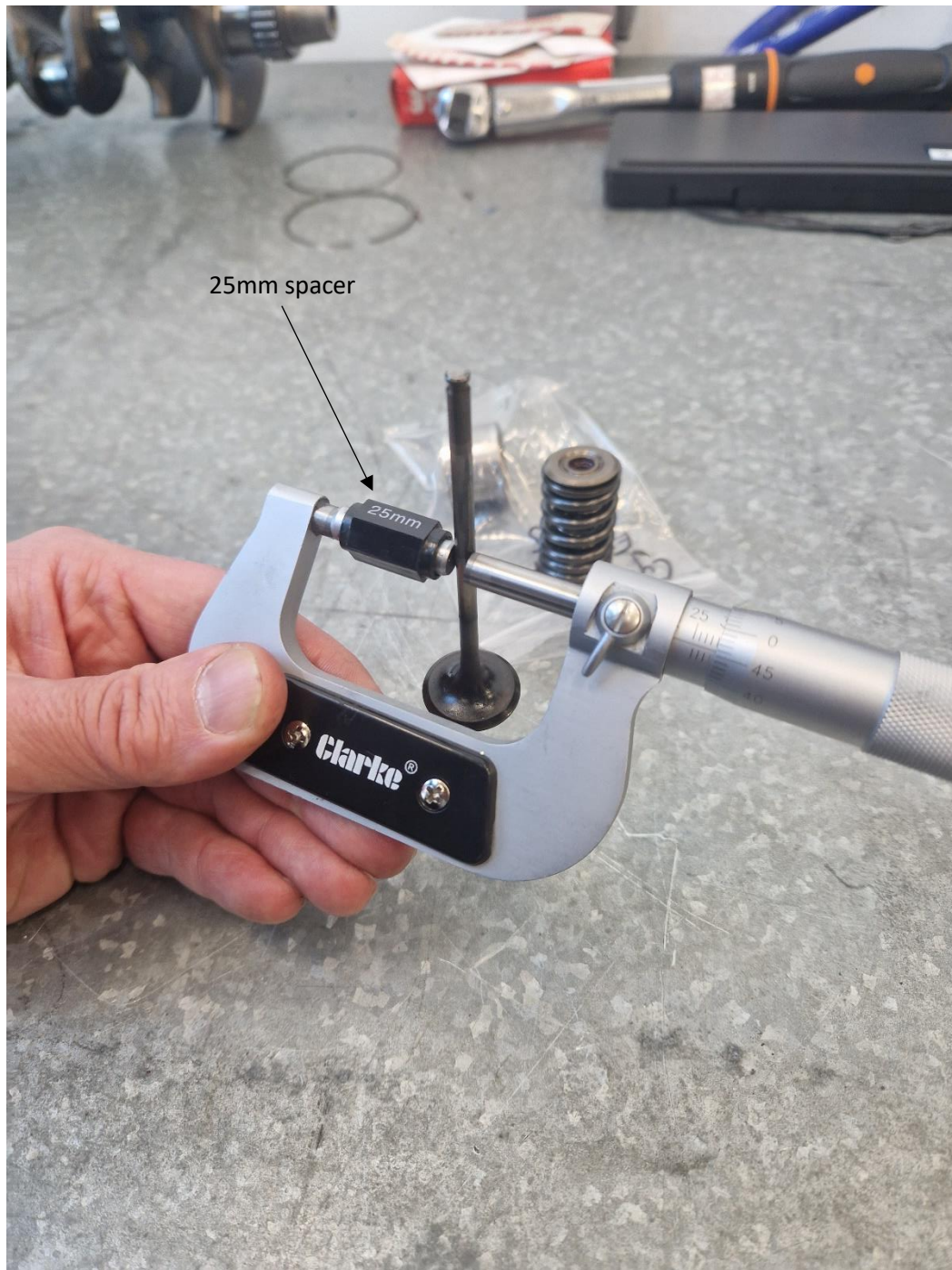
Figure 57: Micrometer measuring valve stem.
