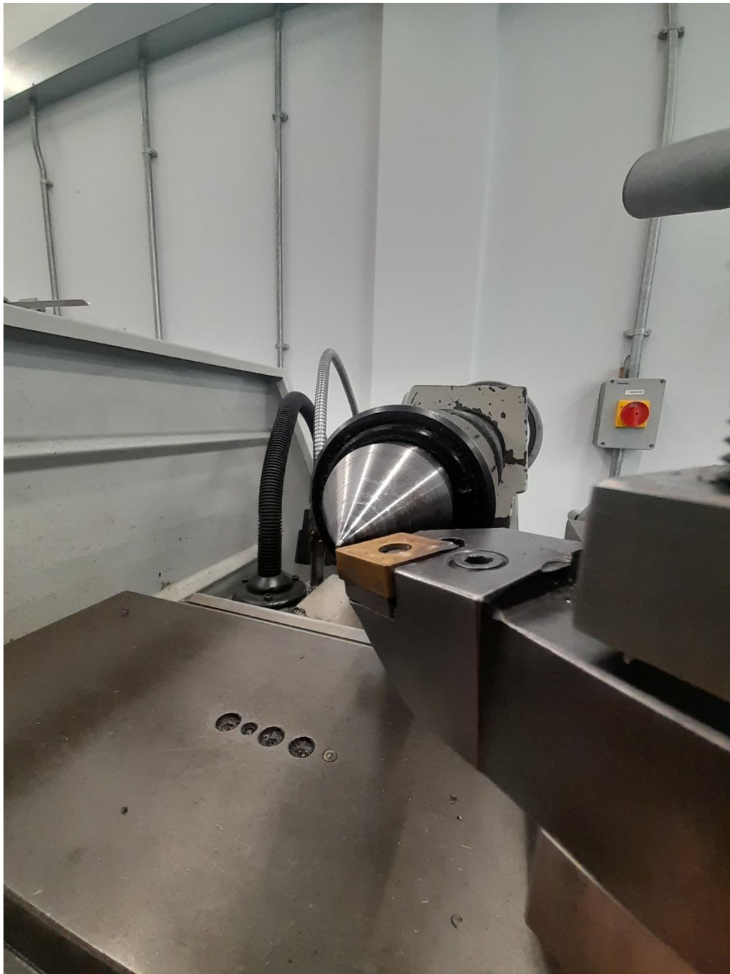
Figure 21: Tool aligned with turning centre.
