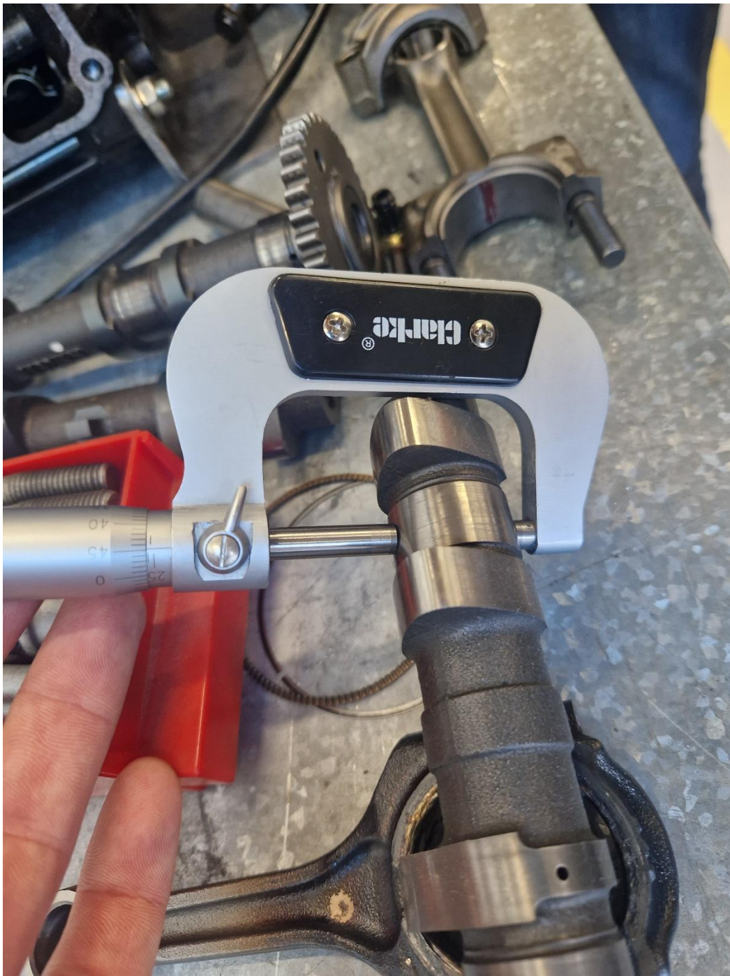
Figure 64: Cam bearing measurement.
