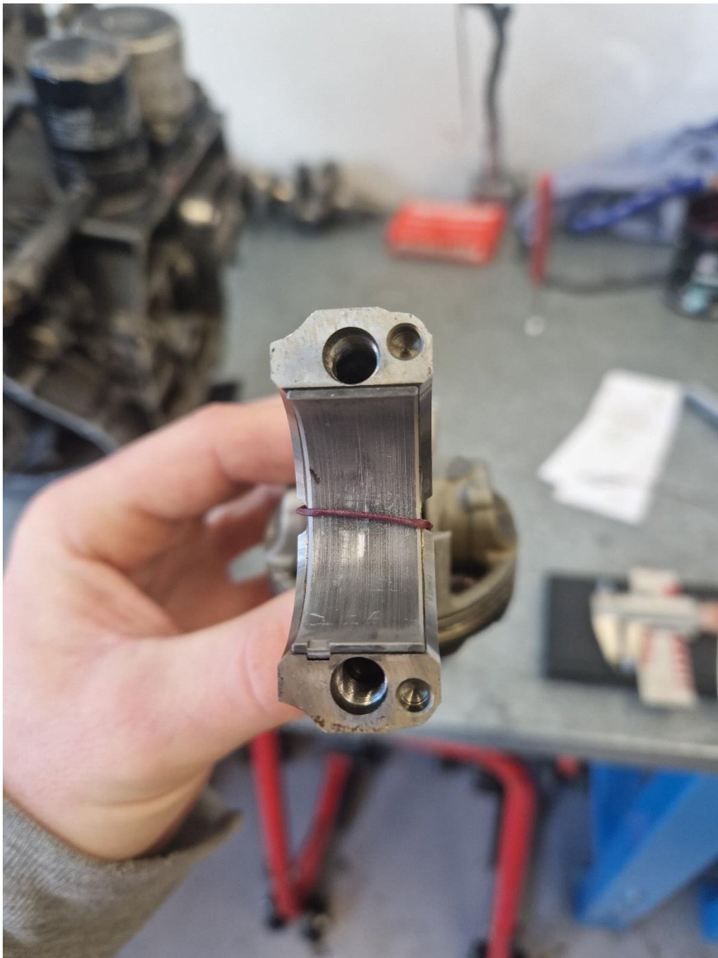
Figure 54: Plastiguage secured to big end of conrod.
