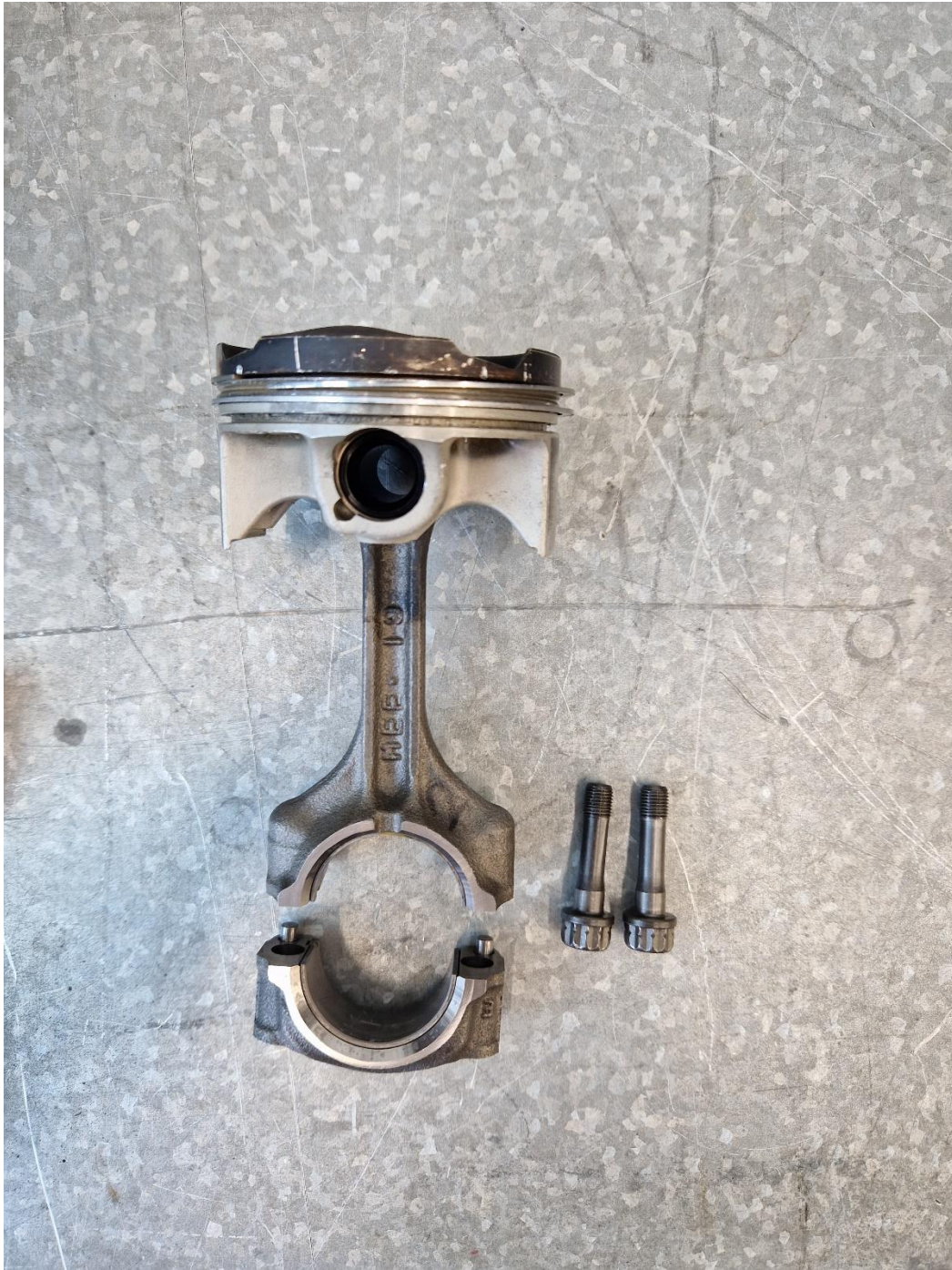
Figure 48: Piston and con rod assembly.
