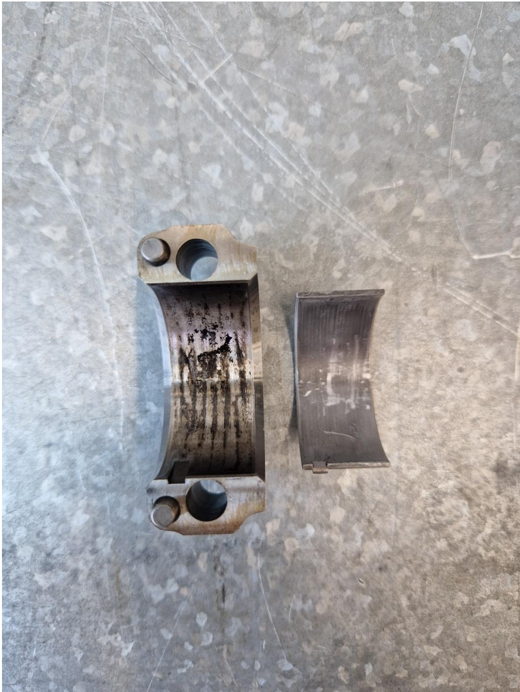
Figure 46: Big end bearing insert removed.
