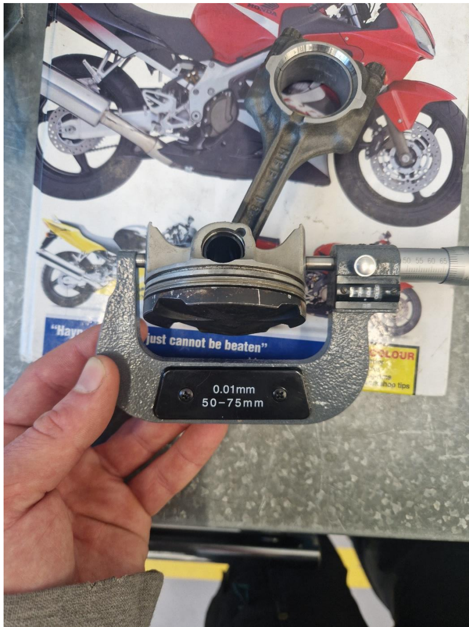
Figure 61: Piston skirt measurment.
