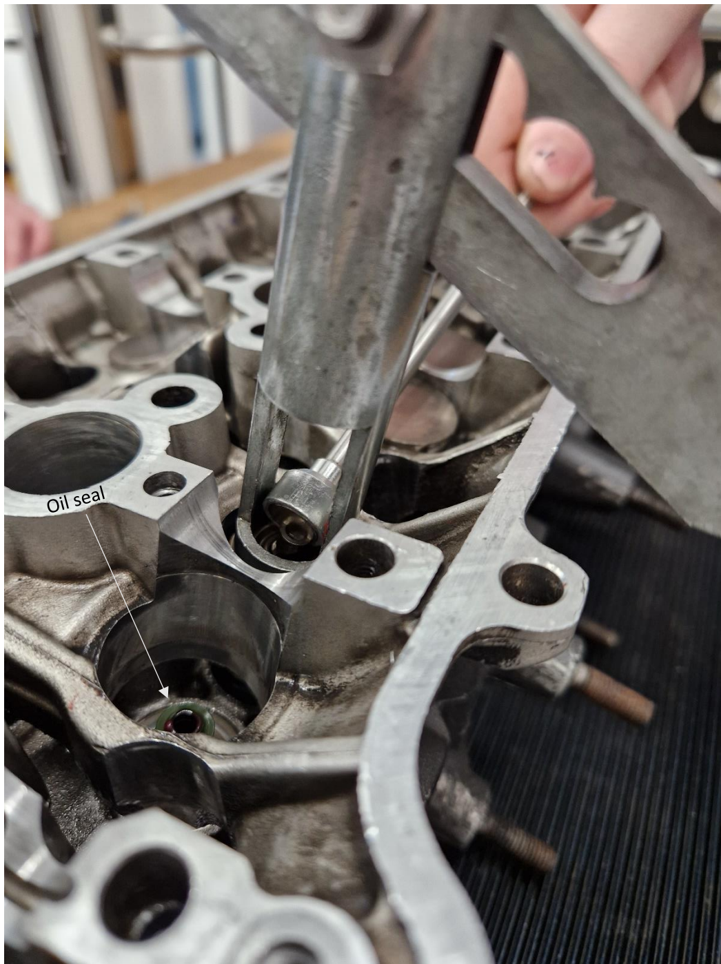
Figure 38: Using a telescopic magnet to remove valve collets whilst spring is compressed.
