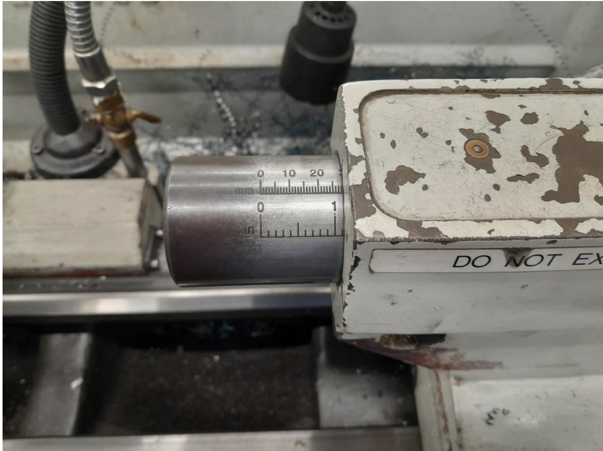
Figure 17: Tail stock wound out past 20mm
