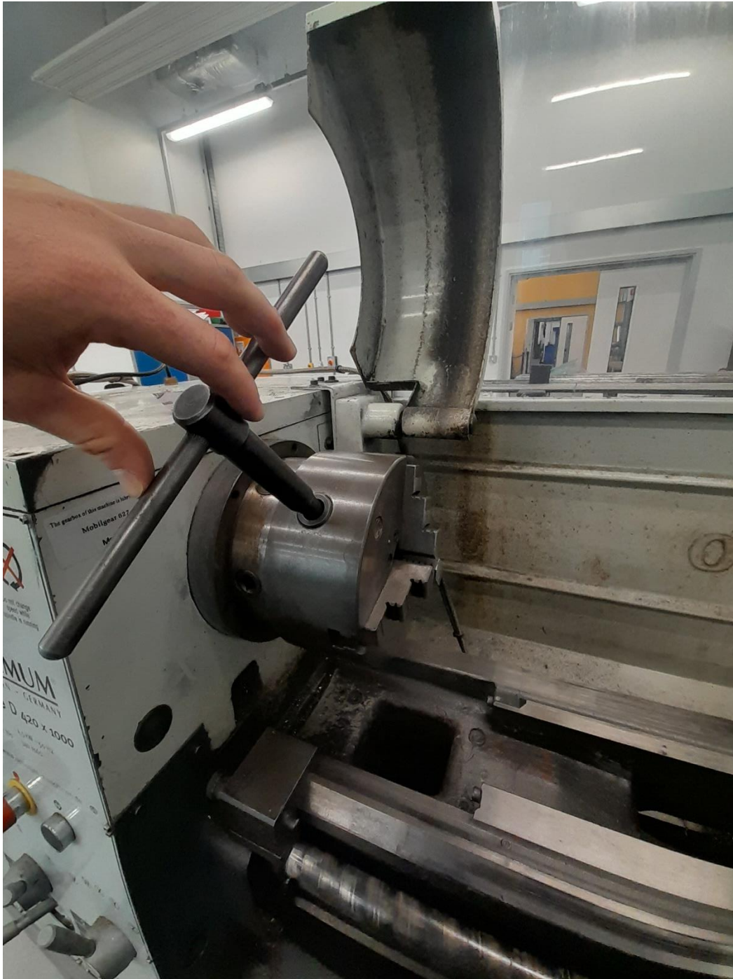
Figure 22: Releasing chuck jaws using chuck tool.
