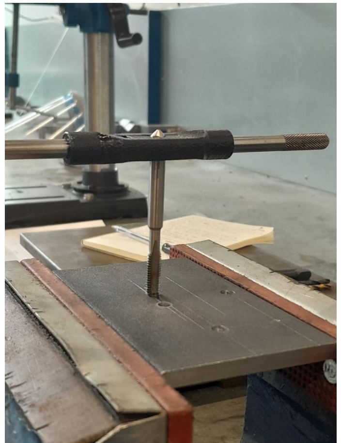
Figure 5: Checking level of tap after first pass.
