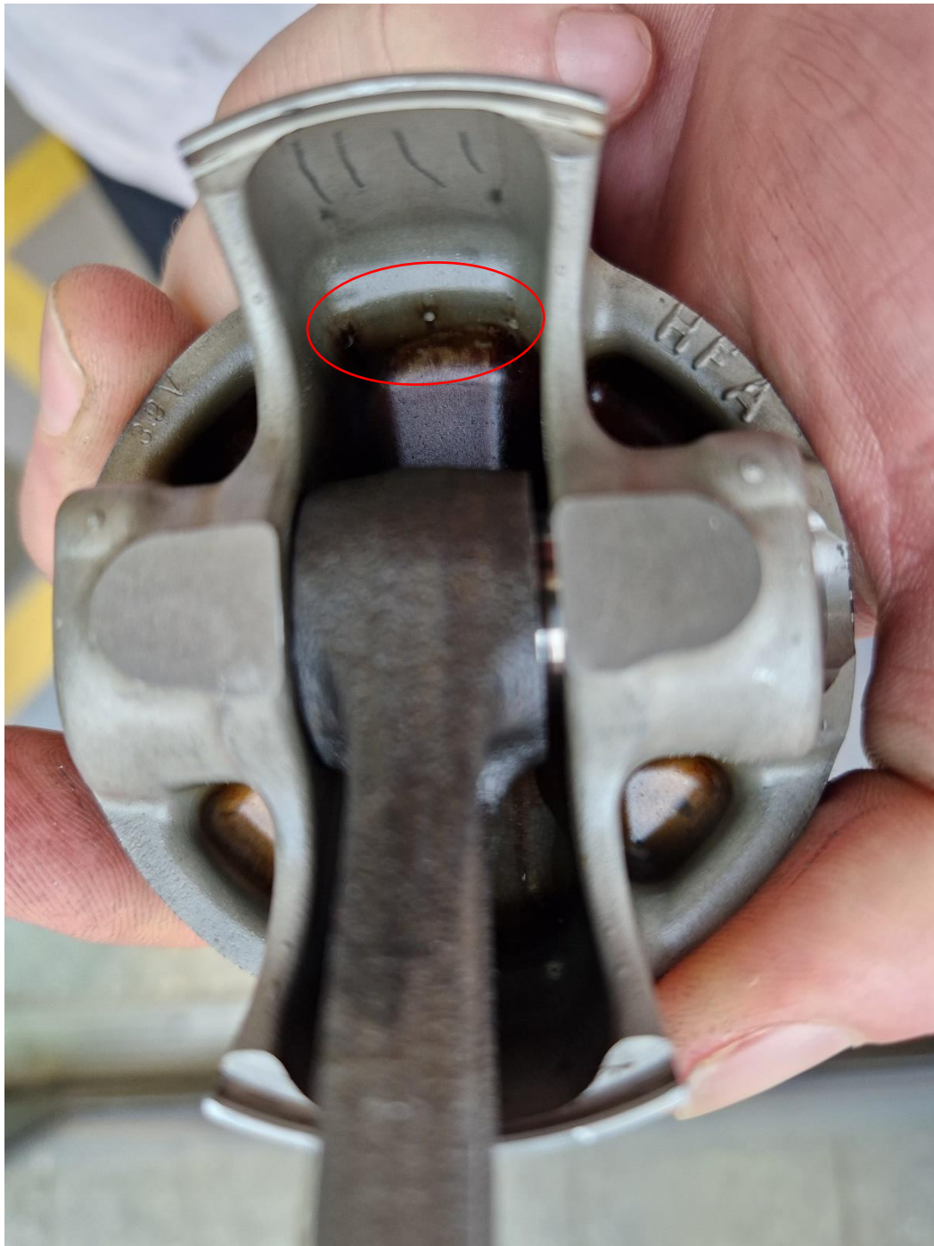
Figure 50: Three oil holes fed from scrape ring circled red.
