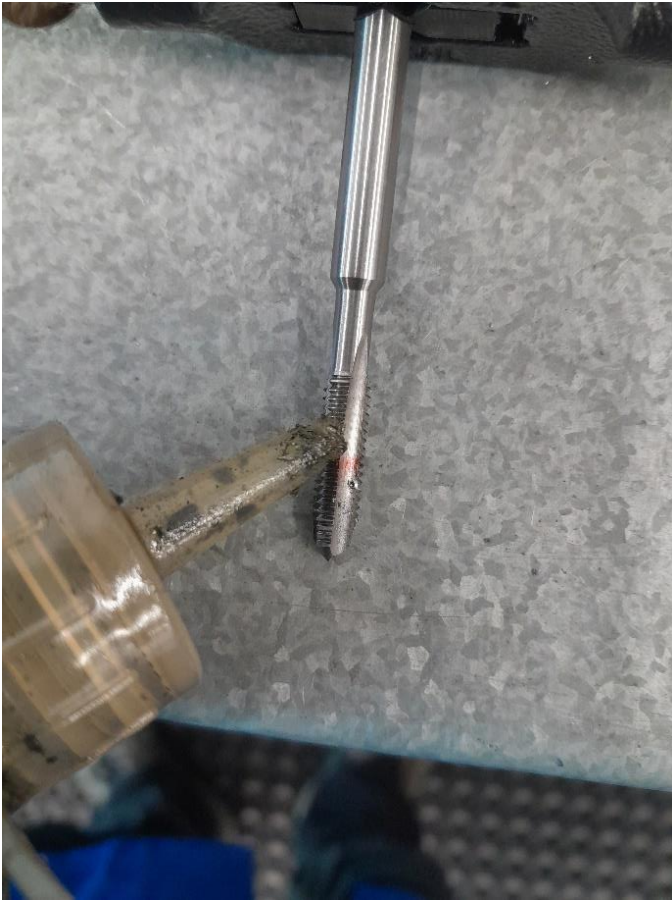
Figure 6: Adding cutting fluid to M6x1.0 tap.
