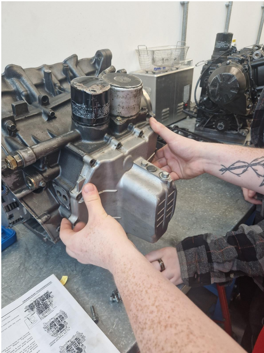
Figure 70: Sump pan installation.
