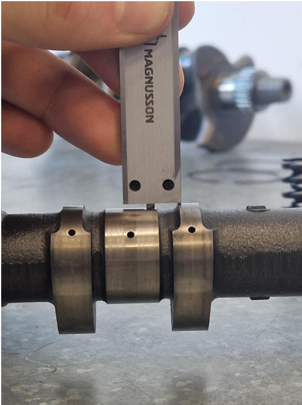
Figure 65: Cam lobe base measurement.
