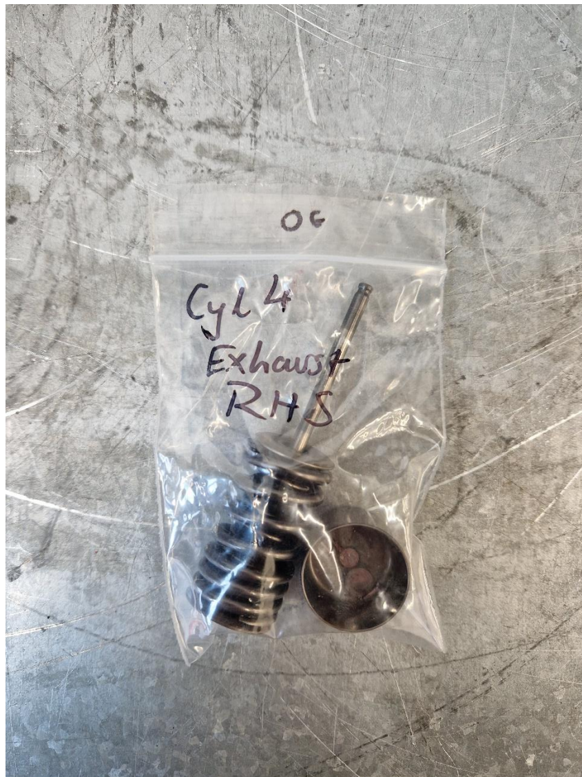
Figure 39: Cylinder 4 right hand side exhaust valve components.
