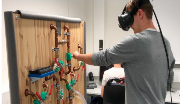
Fig 6. AR hydraulic training rig (Neges, Adwernat and Abramovici, 2018)
