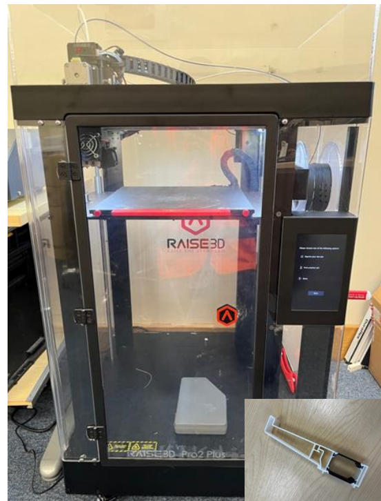
Fig 4. 3D printer and printed prototype at Duraflex window profile manufacturer
