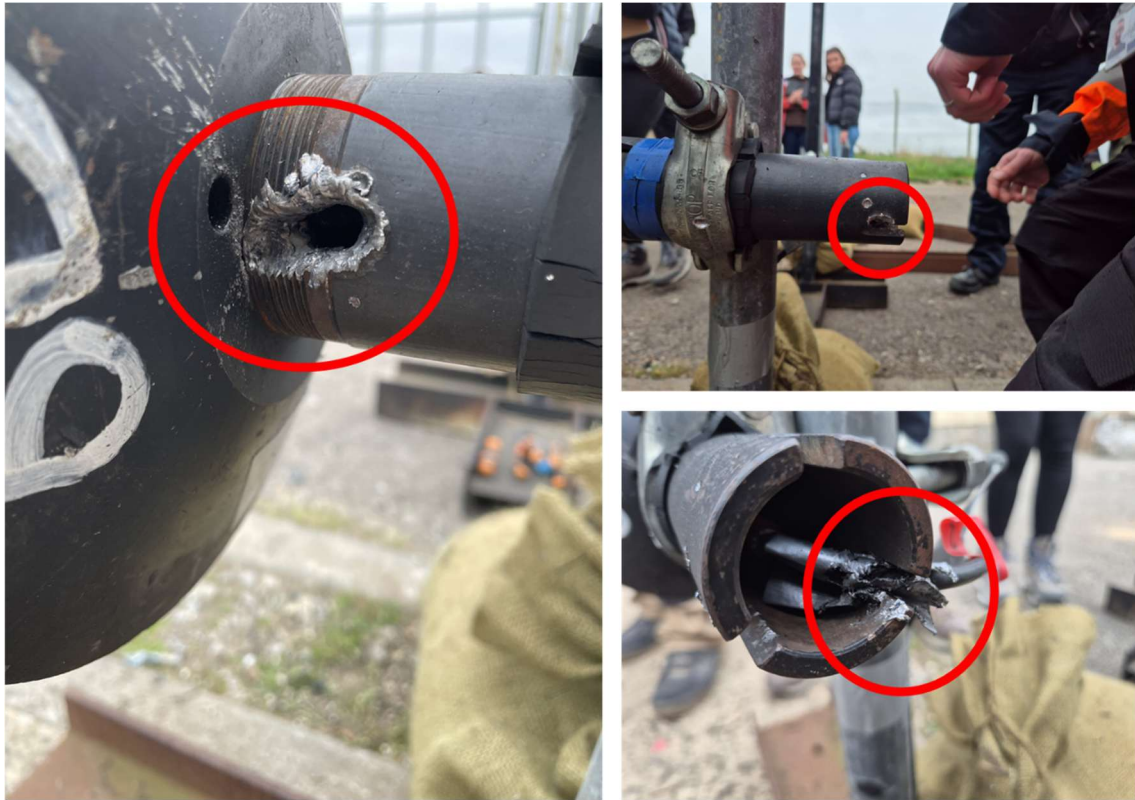
Figure 4-3 - Gauge One Fragmentation Damage from Trial
