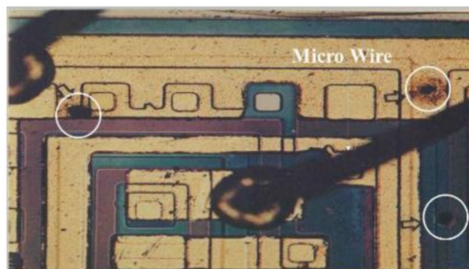
Figure 2.9 - ESD damage on PCB (SlidePlayer, n.d.)
