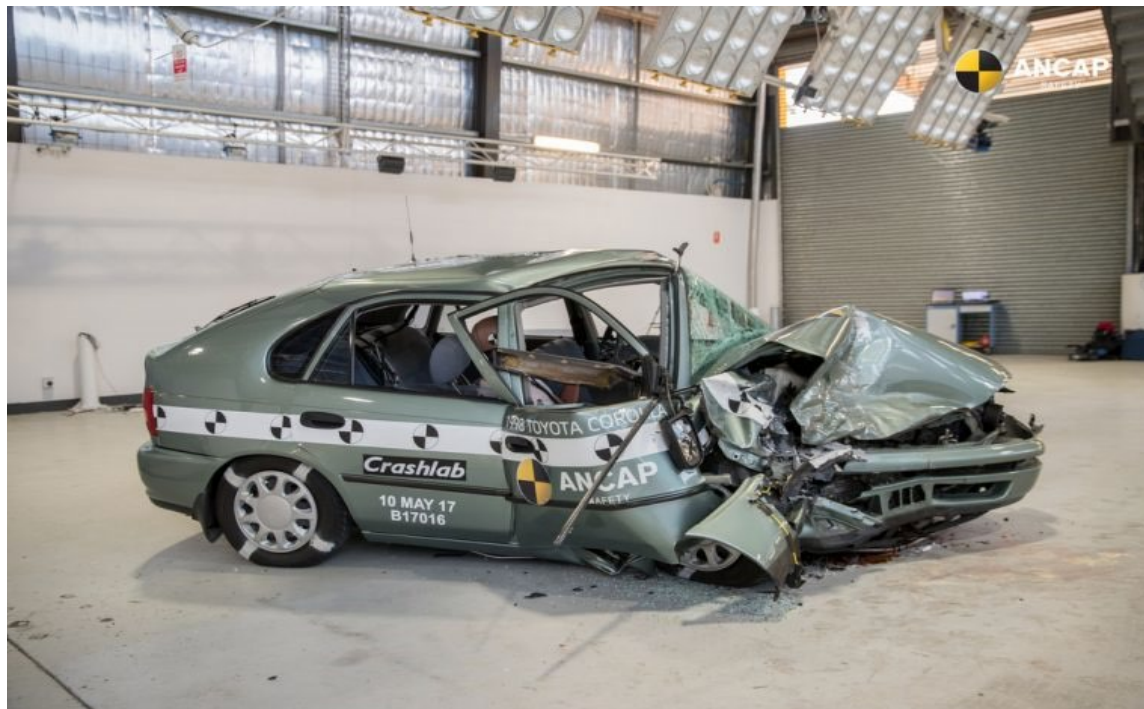
Figure 9: The 1998 Toyota Corolla after impact (Berry, 2017).
