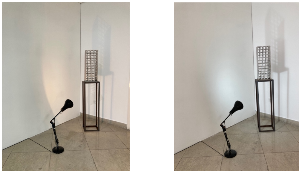
Fig 13. Contrast between light and shadows from the original 40W filament bulb and new 60W LED daylight bulb. Author's images.
