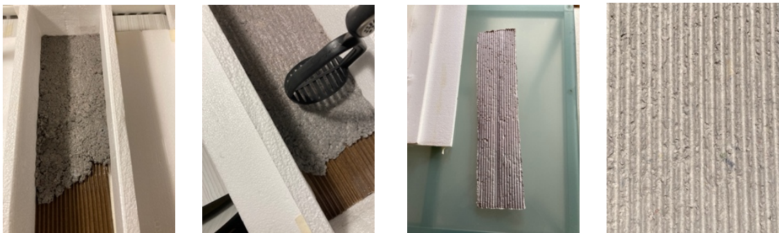
Fig 1. Process of casting newspaper pulp 'concrete' onto corrugated cardboard mould. Author's images.
