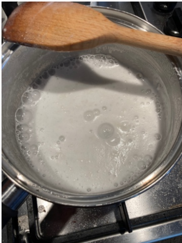
Fig 7. Making and applying casein glue to assemble tower. Author's images.
