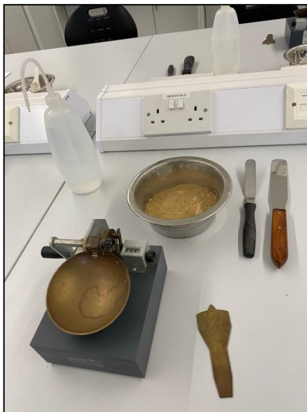
Figure 18: Image showing distilled water, mixing bowl containing the dry soil sample, spatulas, Casagrande apparatus device and groove tool.
