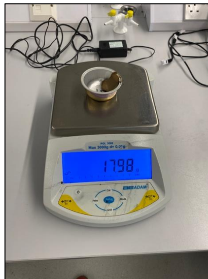
Figure 28: Image of the paste sample being weighed on the precision scales.
