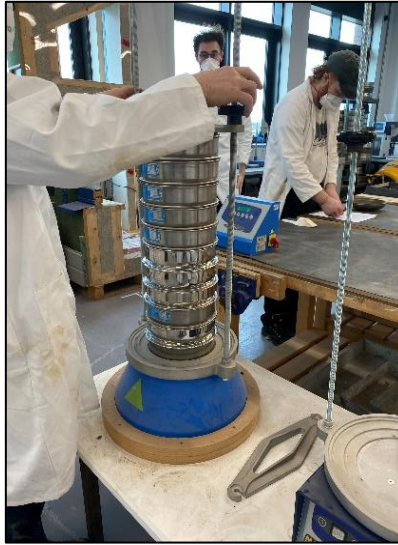
Figure 5: Image of the tightening knobs being secured on the sieve stack lid.
