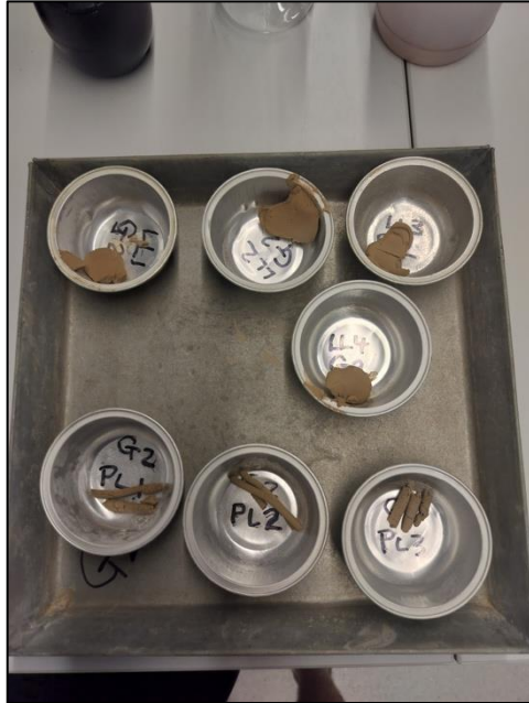
Figure 33: Image of all soil samples in containers after being dried in the oven.
