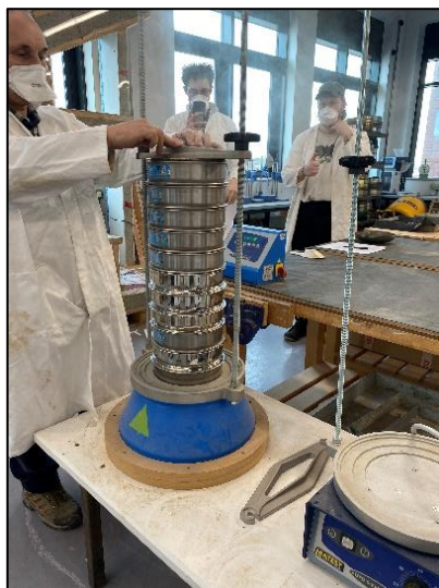
Figure 6: Image of the sieve shaker on with a cloud of dust coming from it.
