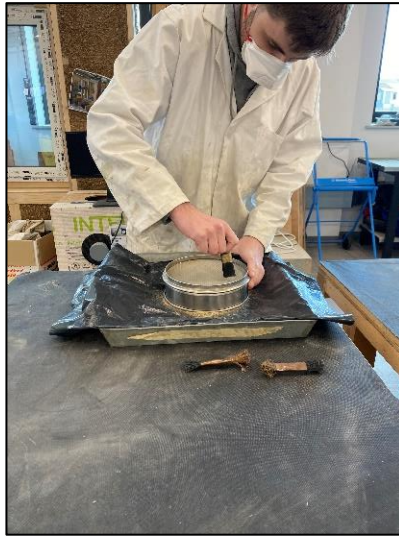
Figure 8: Image of the soil remnants on the sieve being brushed into the collection tray lined with a plastic sheet.
