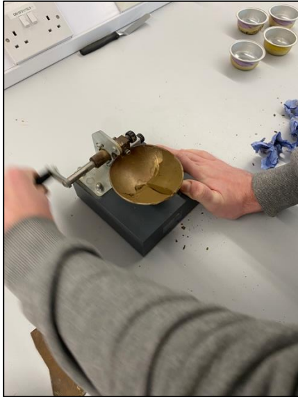
Figure 26: Image of the device handle being rotated while the cup is rising and dropping.
