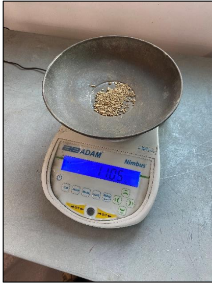
Figure 11: Image of soil collected from a sieve being weighed on a scale.
