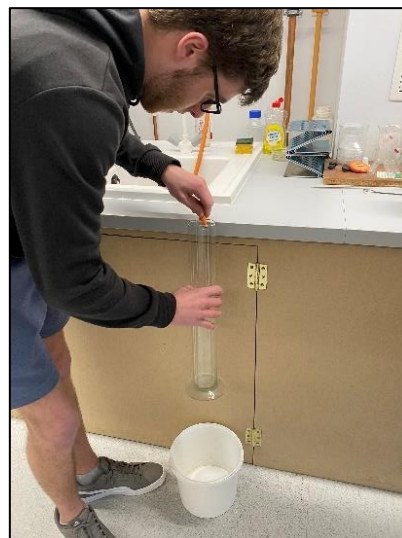
Figure 47: Image of water flowing out of outlet tube into a graduated cylinder whilst being timed.
