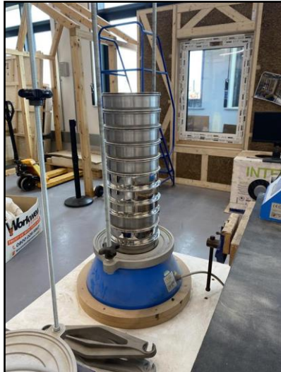
Figure 3: Image of the 10 test sieves stack with the largest sieve size on top, and the smallest on the bottom.
