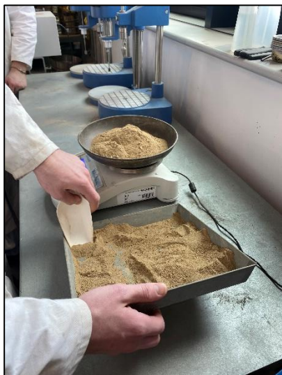
Figure 2: Image of the soil sample being scooped into the scale pan.
