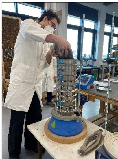
Figure 4: Image of the soil sample being poured into the top sieve on the stack.
