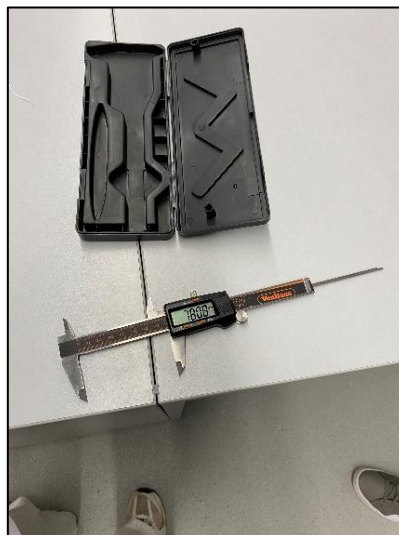
Figure 40: Image of digital vernier calliper after taking measurement of internal diameter of constant head permeameter.
