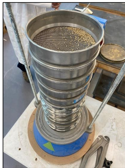
Figure 7: Image showing the soil granules collected by the top sieve after vibration.
