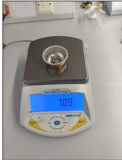
Figure 34: Image of a dry PL soil sample and container being weighed on precision scales.
