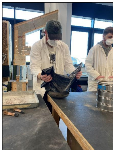
Figure 9: Image of the soil granules being transferred into the scale pan via a plastic sheet.
