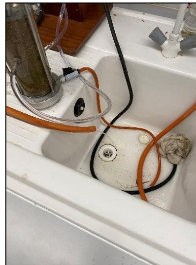
Figure 43: Image of water flowing out of constant head permeameter via outlet tube.
