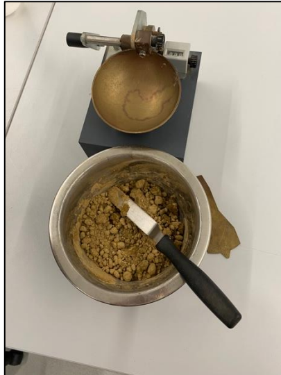
Figure 22: Image showing some distilled water mixed into the soil sample.
