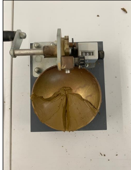
Figure 27: Image showing the groove has closed.
