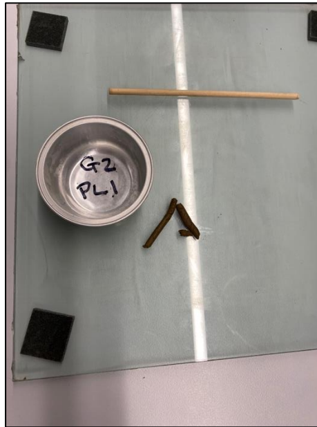
Figure 31: Image of the crumbled soil thread against the wooden rod.
