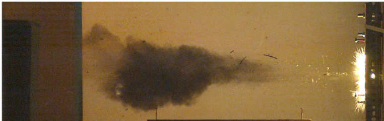
Figure 15 - Snapshot of high-speed imagery from firing 3 showing flash from copper impact
