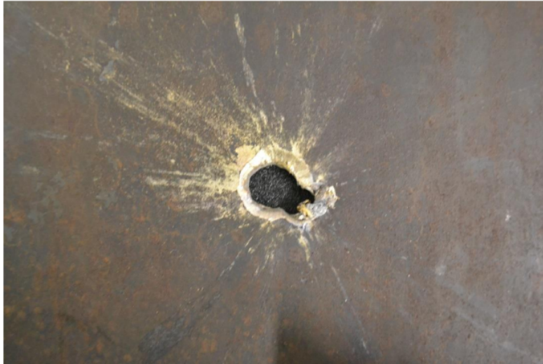
Figure 24 - Presence of gold coloured compound on rear of target plate
