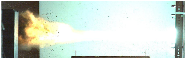
Figure 14 - Snapshot of high-speed imagery to show aluminium flash upon impact from firing 8
