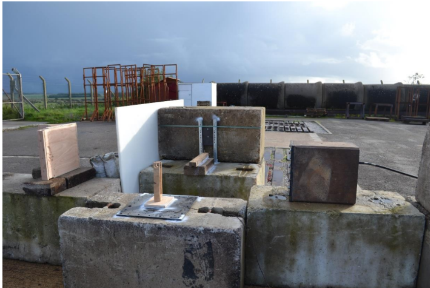
Figure 8 - Experimental set-up detailing charge stand position (centre), flash x-ray head position (Right) and x-ray cassette position (Left)
