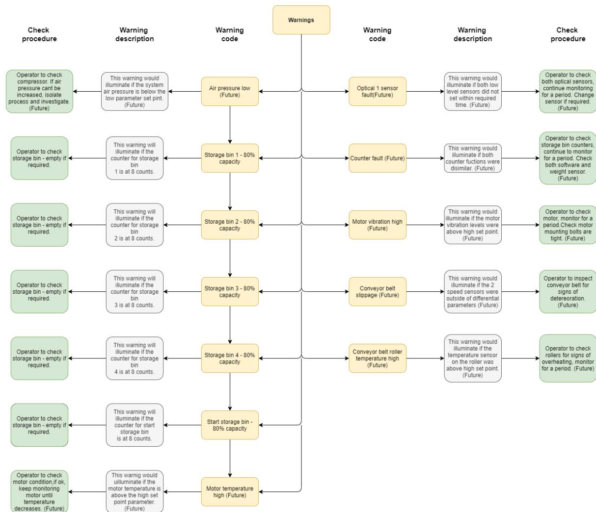
Figure 35 - Warnings audit and check
