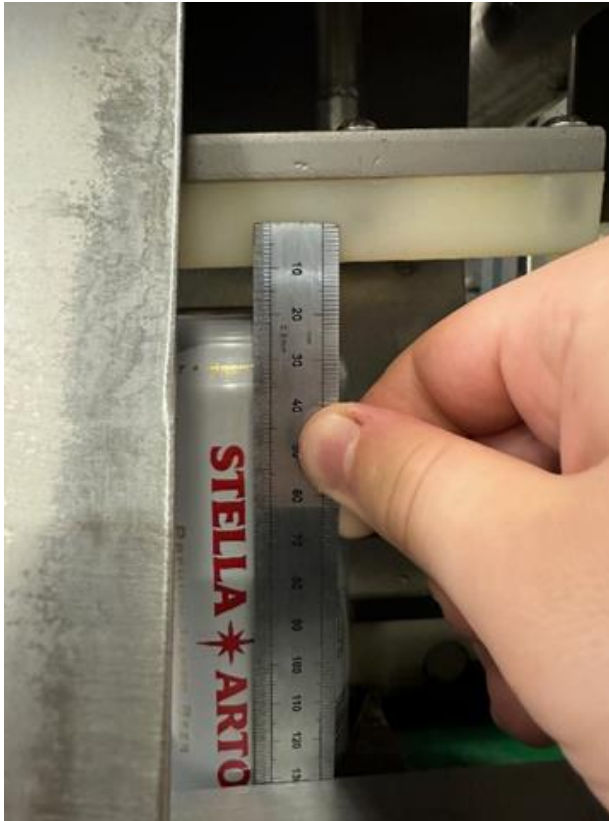
Figure 2 – Setting Bubble Breaker Block Height with Stainless Steel Rule
