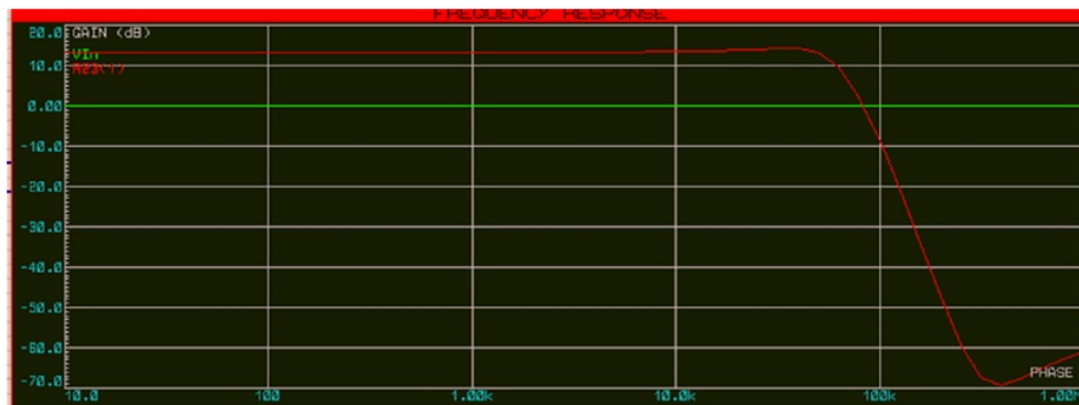
Figure 11: Frequency Graph of a Sixth Order Low Pass Filter
