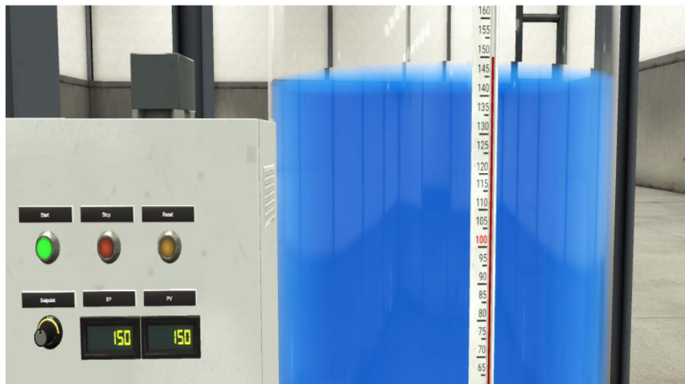
Figure 7; Test - Fill to 150, Check Panel PV display
