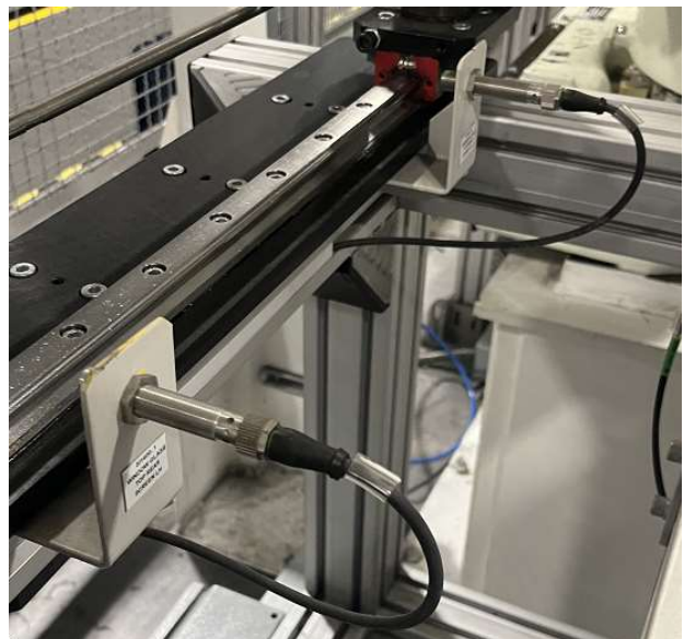
Figure 3 – Proximity sensors detecting clamp positions
