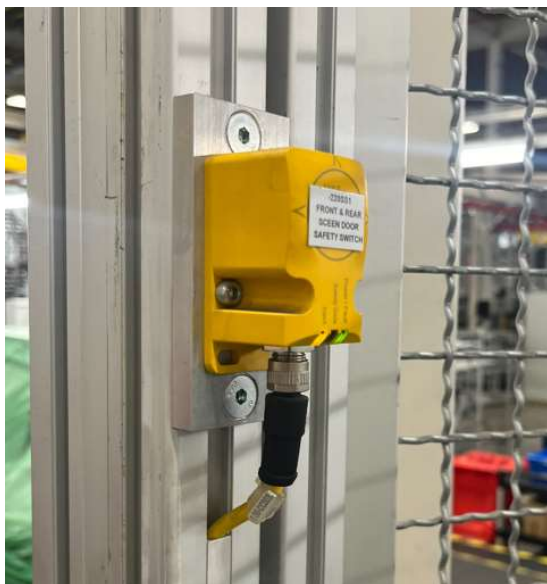
Figure 2 – Proximity sensor for gate detection
