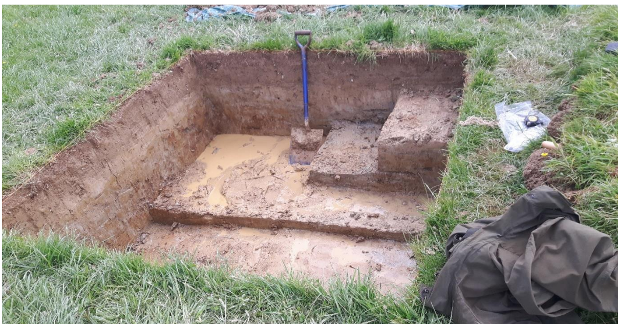
Image 6 & 7 Test pit hand dug with formed steps, continued water ingress determined form of test pit.
