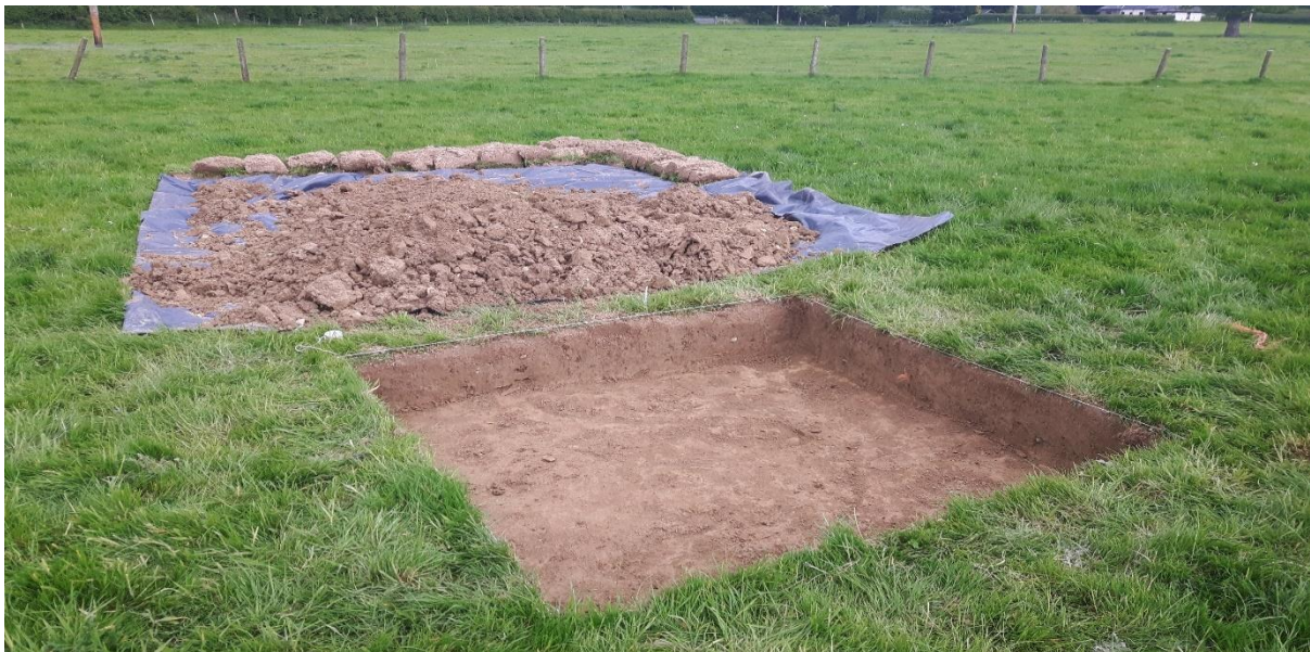
Image 6 & 7 Test pit hand dug with formed steps, continued water ingress determined form of test pit.
