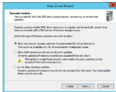
Figure 118: Secure dynamic update selected (AD) for periodic update of secondary DNS zone (Swansea)
