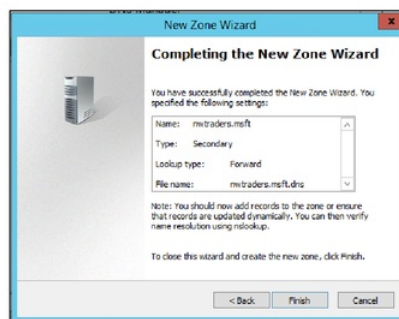
Figure 109: Configuration review and secondary forward zone created
