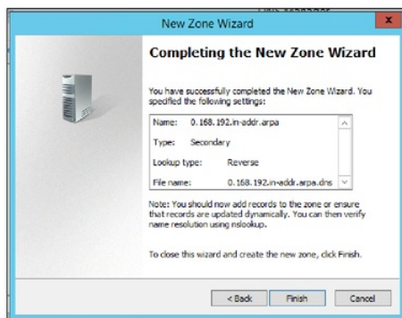
Figure 115: Reverse lookup zone configuration confirmation and creation
