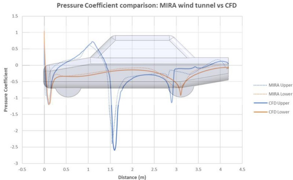
Figure 15. Pressure coefficient comparison of MIRA wind tunnel data to CFD data
