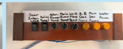
Figure 5 - Controls for thermocouples, pressure gauges, door interlock and pressure relief panel
